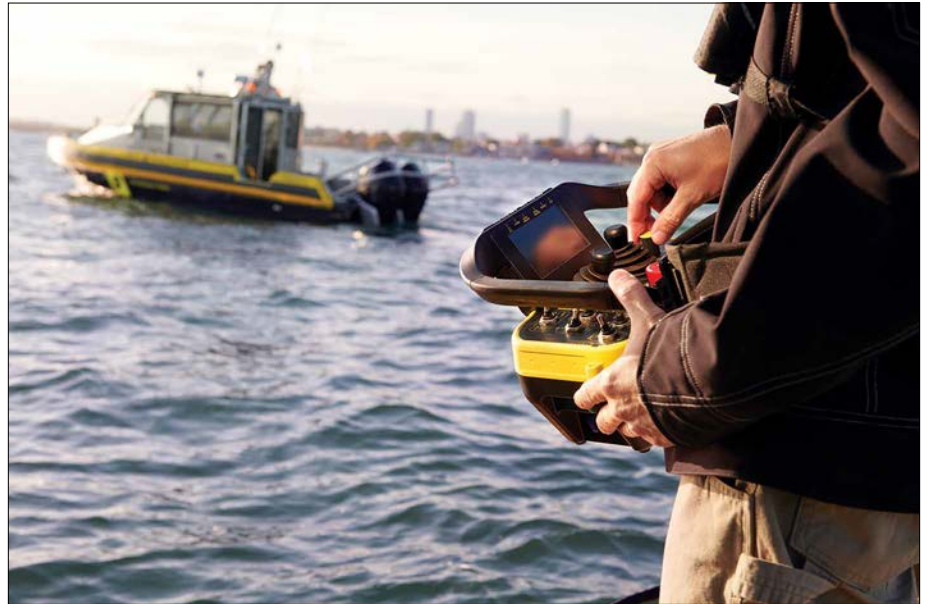
The Sea Machines SM200 system enables wireless helm and propulsion control, as well as remote control of auxiliaries and payload equipment. The Coast Guard and the American Bureau of Shipping approved the SM200 in early 2020 for installation aboard a class of U.S.-flag tugboats that support articulated tug-barge sets. Photo courtesy of Sea Machines
