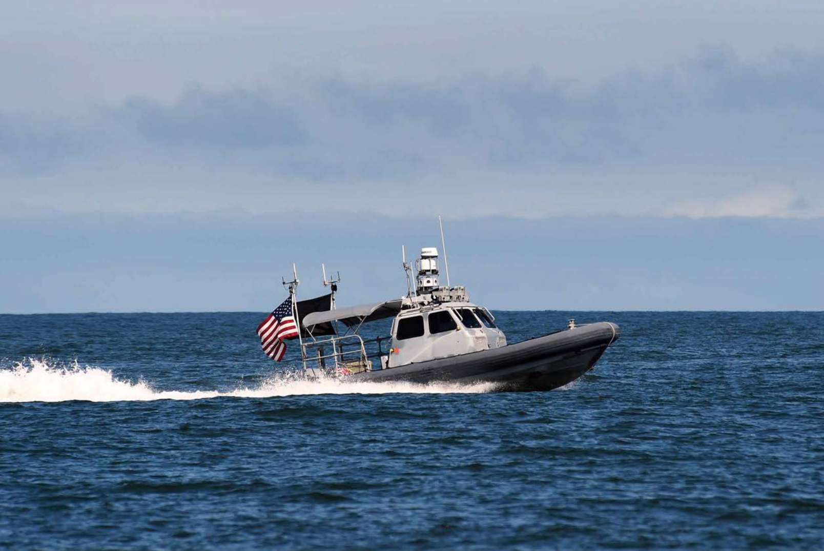
An unmanned rigid-hull inflatable boat operates autonomously during an Office of Naval Research-sponsored demonstration of swarmboat technology at Joint Expeditionary Base Little Creek-Fort Story, Virginia, in September 2016. Navy photo by John F. Williams
