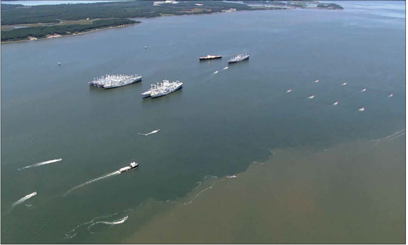
Eight unmanned high-speed maneuvering surface targets, upper right, lead the way as five unmanned autonomous vehicles escort a high-value asset during an Office of Naval Research-sponsored demonstration of autonomous swarmboat technology on the James River in Newport News, Virginia, in 2014. U.S. Navy photo
