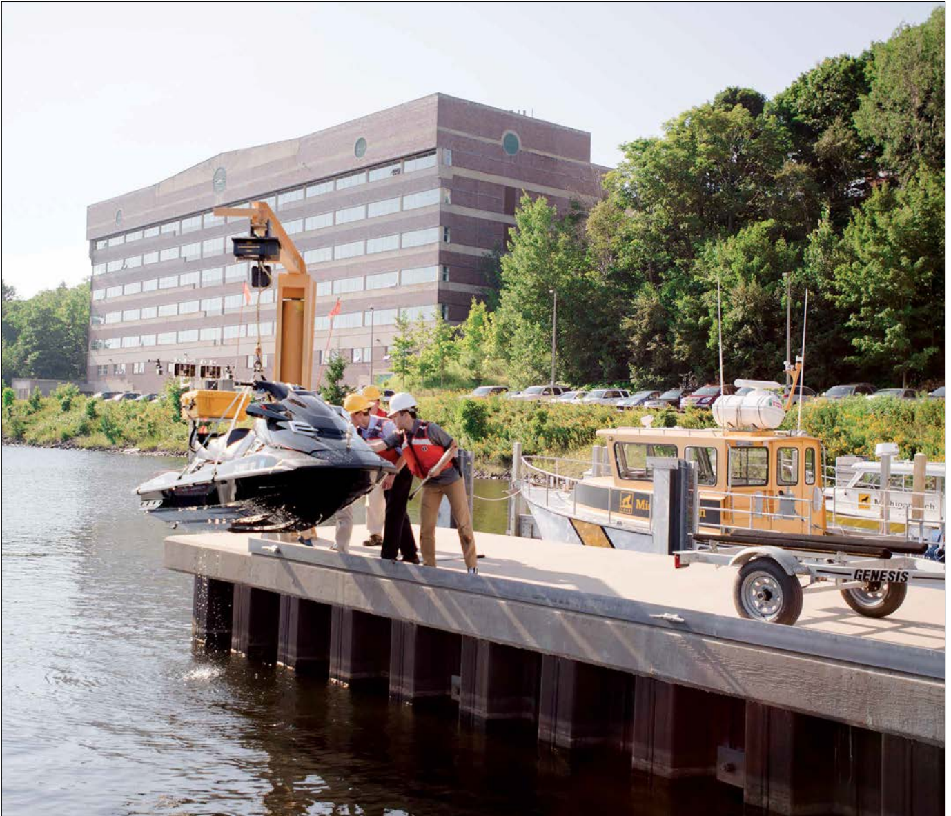
Engineering students deploy an autonomous surface vehicle built upon a stock Yamaha WaveRunner personal watercraft at the Marine Autonomy Research Site in Michigan's Upper Peninsula. Photo courtesy of Michigan Technological University
