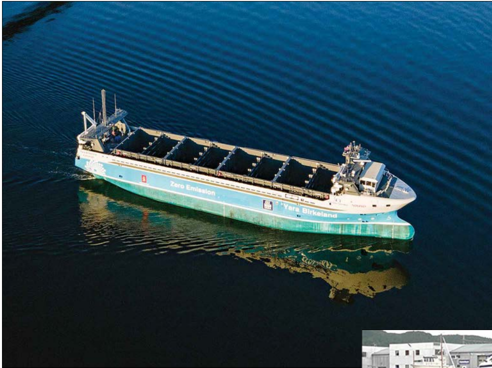
The Yara Birkeland , left, sails through Brevik, Greenland Harbour, Norway, on its way to Norwegian shipyard Vard Brattvåg on its first autonomous voyage in 2020. Upon delivery, the vessel will be tested for container loading and stability before undergoing further preparations for complete autonomous shipping. Photo courtesy of Knut Brevik Andersen of Wilhelmsen Ship Service Below, Norwegian University of Science and Technology researchers collect data while testing the autoferry prototype on Norway's Trondheim Canal in 2018. Photo courtesy of Norwegian University of Science and Technology
