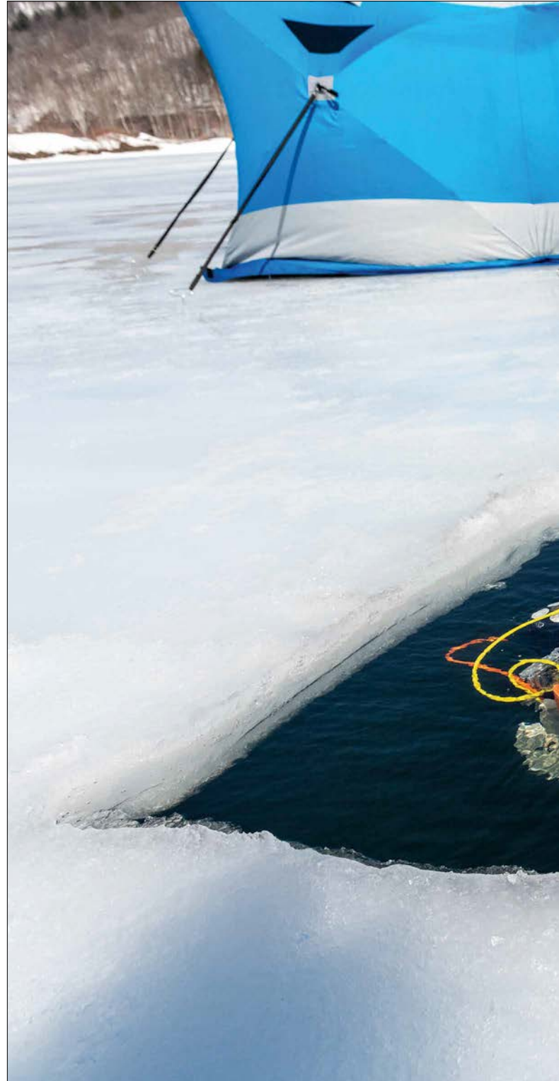
A remotely operated underwater vehicle is deployed through several feet of Lake Superior ice to evaluate future Arctic capability. Photo courtesy of Michigan Technological University
