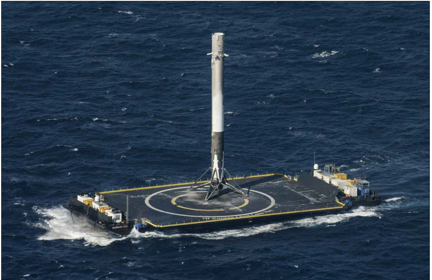
The first stage of a Falcon 9 Full Thrust rocket lands on the autonomous spaceport drone ship Of Course I Still Love You in 2016. The Coast Guard is currently negotiating a design basis agreement that will use autonomous technology to facilitate rocket-recovery missions on board a Subchapter I vessel. Photo courtesy of SpaceX
