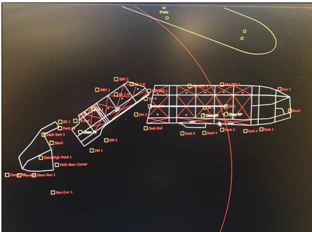
A schematic of the ship, Coimbra , clearly outlines the three large sections remaining after its sinking. Coast Guard graphic
