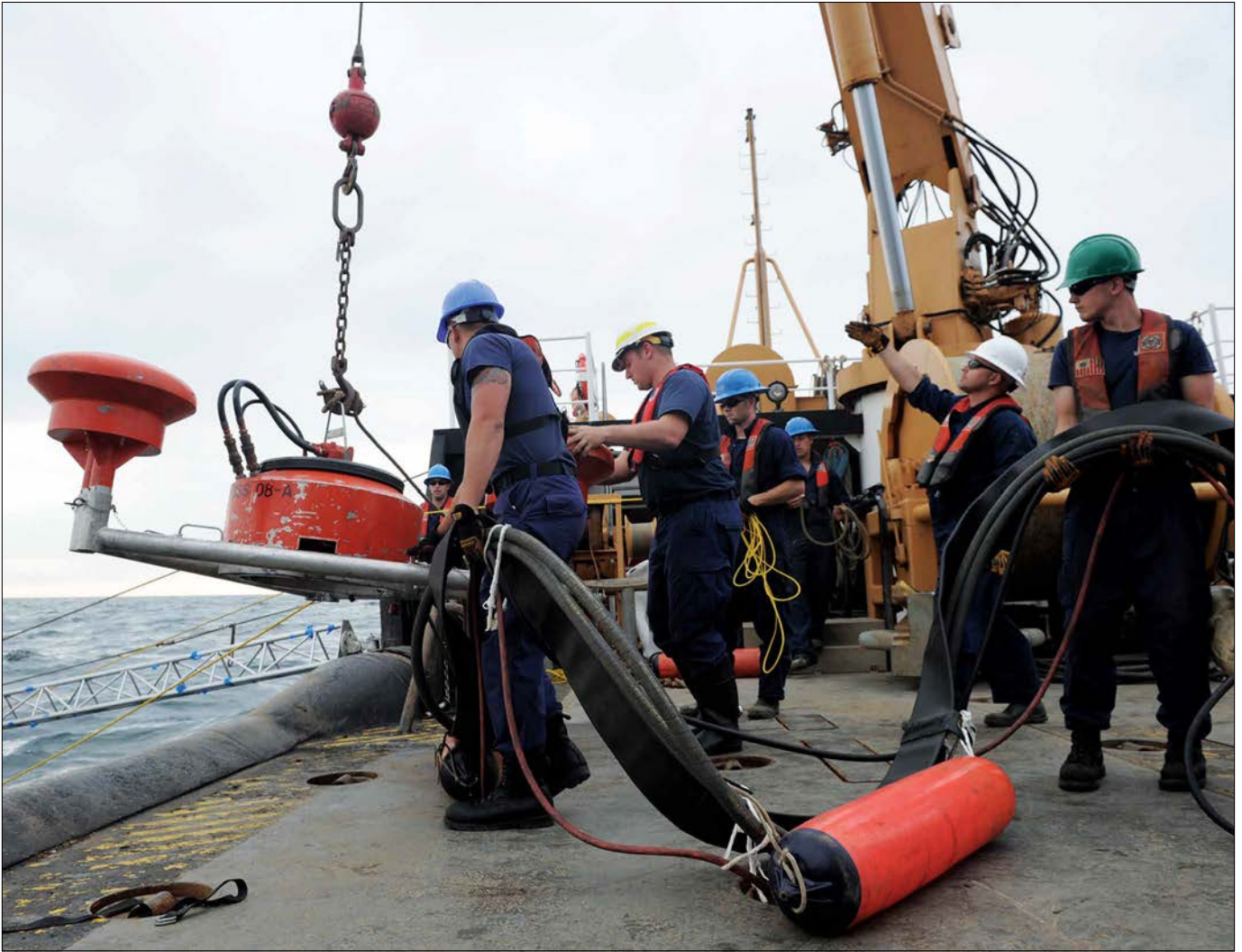
Crew members from the Coast Guard Cutter Harry Claiborne work to move a vessel of opportunity skimming system into the Gulf of Mexico in May 2010. The Coast Guard worked in partnership with BP, local residents, and other federal agencies to help keep the oil from spreading after the Deepwater Horizon explosion on April 20, 2010. U.S. Navy photo by Petty Officer 2nd Class Jonathen E. Davis
