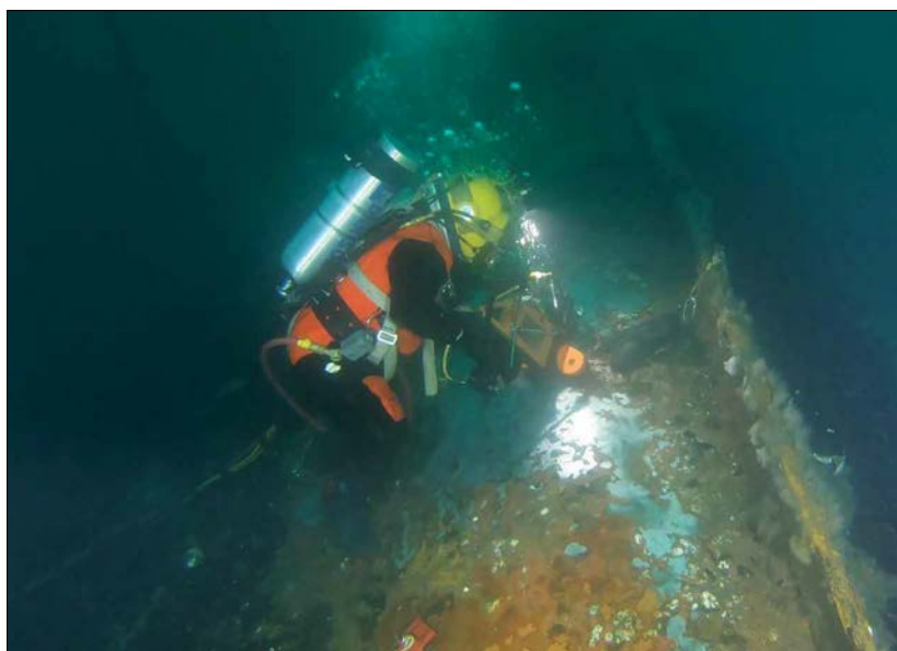
Divers securely drill into the oil tanks of British-flagged tanker Coimbra , May 8, 2019. The tanker was torpedoed by a German U-boat during World War II. Coast Guard photo
