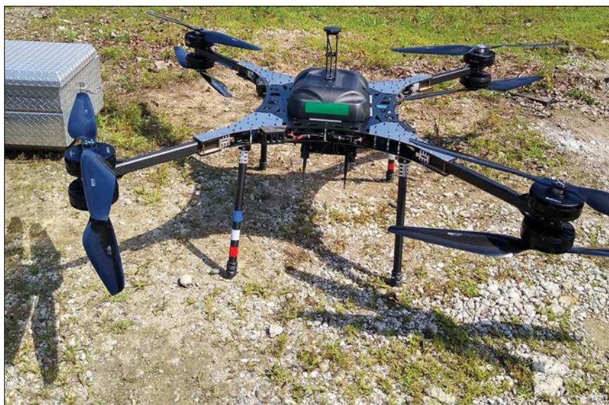
The Hx8 XXL is an American-made unmanned aviation system, used in a Defense Logistics Agency operation to carry supplies to the Coast Guard Cutter Lawrence O. Lawson . It can carry payloads of up to 70 pounds for up to 5 miles. Coast Guard photo by CWO4 Todd Wardwell
