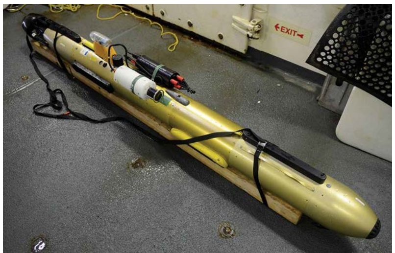
A Gavia Scientific autonomous underwater vehicle (AUV) dries on the deck of the Coast Guard Cutter Healy after recovery from a simulated oil in ice exercise in the Arctic in August 2014. The AUV is outfitted with sonar and radar sensors that allow responders to locate oil trapped beneath or within the ice. Coast Guard photo by Petty Officer 1st Class Shawn Eggert
