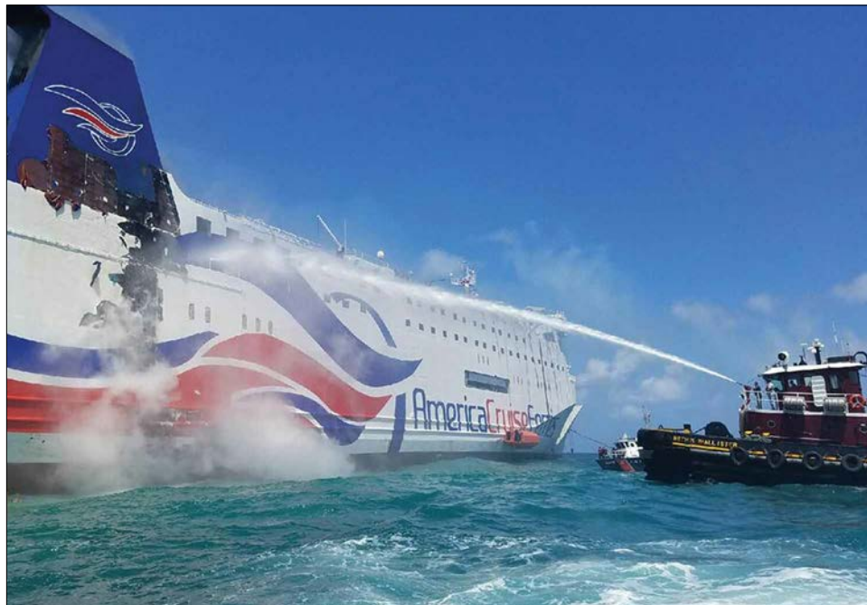
A local San Juan, Puerto Rico-based tug crew uses a fire hose to cool the hull of the 614-foot Caribbean Fantasy after its engine room caught fire on August 17, 2016. The fire began to spread forcing passengers and crew to abandon the vessel a mile from San Juan Harbor, Puerto Rico. Coast Guard photo
