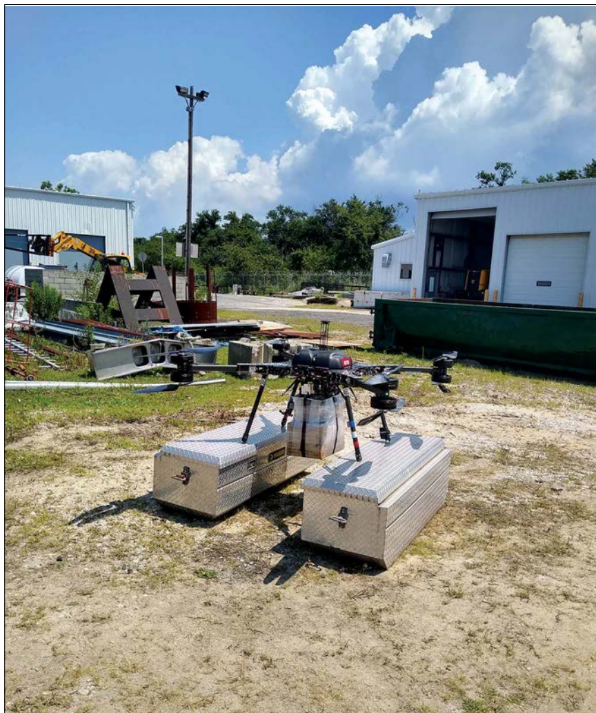
The Hx8 XXL unmanned aviation system is shown here, loaded and ready to fly, with over 60 pounds of Meals Ready-to-Eat, and two cases of bottled water underslung from its cargo system. This was part of a joint exercise between the crew of Coast Guard Cutter Lawrence O. Lawson and the Defense Logistics Agency. Coast Guard photo by CWO4 Todd Wardwell
