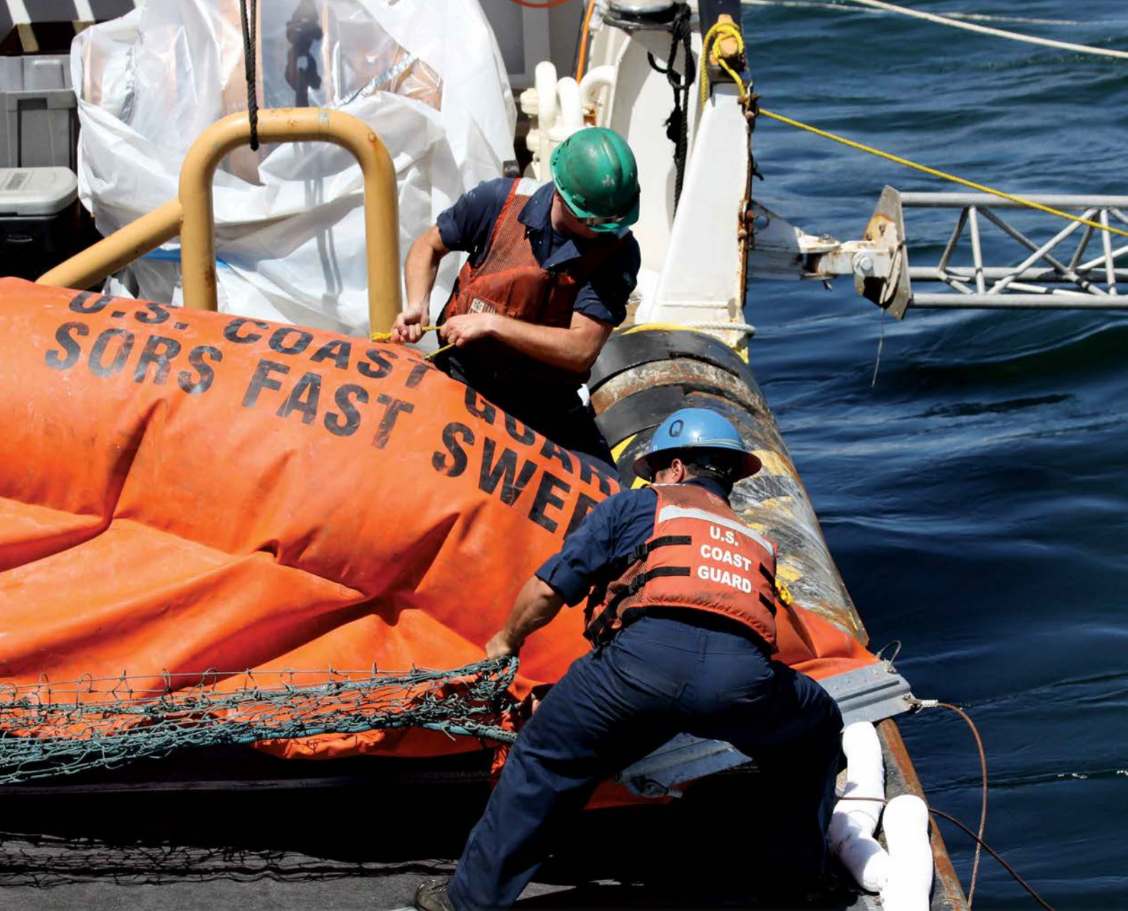
Two crew members from the Coast Guard Cutter Walnut haul a spilled oil recovery system across the cutter's buoy deck for deployment. The floating fast-sweep boom collects oil alongside the cutter for skimming and containment in tanks on its deck. Coast Guard photo
