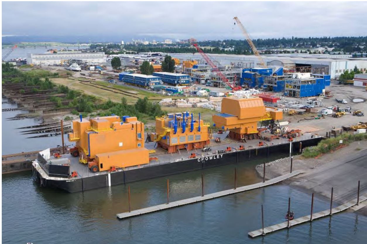
Doyon Drilling Rig 25 shown on the barge in the foreground. Due to the size of the rig and its six mega-modules, two barges were required for delivery to Alaska's North Slope. The background shows the remaining modules for Rig 25, in addition to Parker Drilling's AADU Rigs (Rig 272 and Rig 273)
