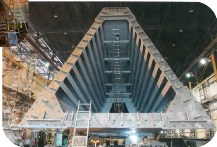
The lower segment of the iconic Portland Aerial Tram's tower is shown inside Thompson Metal Fab's shop. Including the bunking underneath, the tower is nearly 40' high and 30' wide. The completed tower can be seen at OHSU, spanning over I-405.
