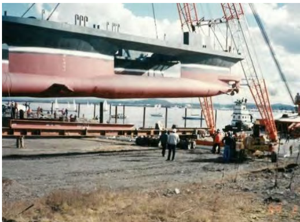
These structures are 9' diameter x 132' long and part of a Small Waterplane Area Twin Hull (SWATH). Once assembled in Thompson's yard, the hull measured 53' wide and nearly 60' high once outfitted with the superstructure. Thompson's location adjacent to the Columbia River was a key part in earning this business. After testing in the river, the "Navatek" shipped to Hawaii where the vessel still operates.
