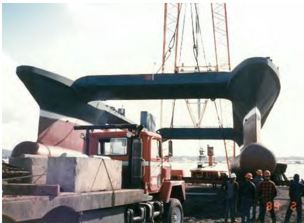
These structures are 9' diameter x 132' long and part of a Small Waterplane Area Twin Hull (SWATH). Once assembled in Thompson's yard, the hull measured 53' wide and nearly 60' high once outfitted with the superstructure. Thompson's location adjacent to the Columbia River was a key part in earning this business. After testing in the river, the "Navatek" shipped to Hawaii where the vessel still operates.
