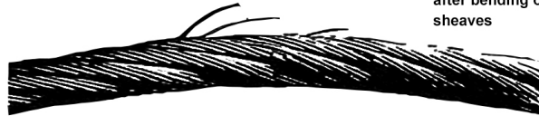
Rope break due to excessive strain
