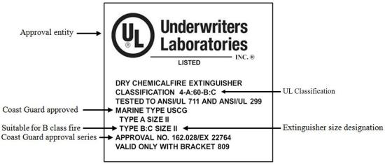
Sample labeling on a B-II fire extinguisher
