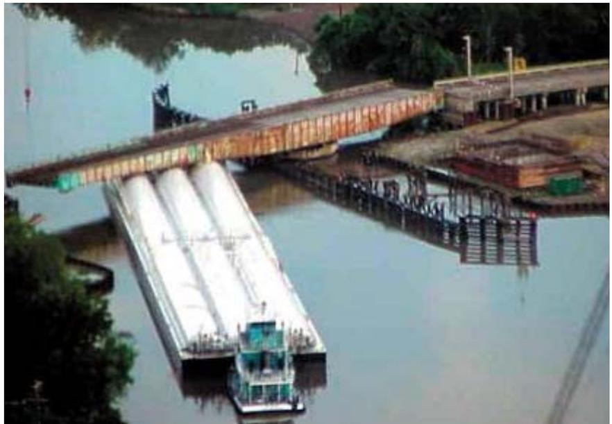
The primary causal factor associated with these casualties was the lack of accurate air draft data for either the towing vessel or its tow being made available to the responsible Master or Mate. Knowledge of a vessel's air draft is a critical component in determining whether a vessel can pass safely under a bridge or overhead structure.
