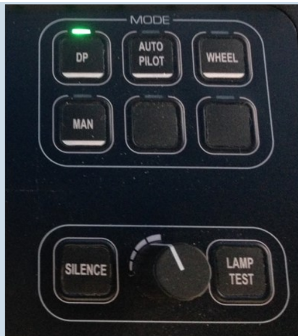
Figure 1: The “Man” and “Silence” buttons are roughly ¼ of an inch apart. Also, white lines on buttons require double push within 5 seconds.
