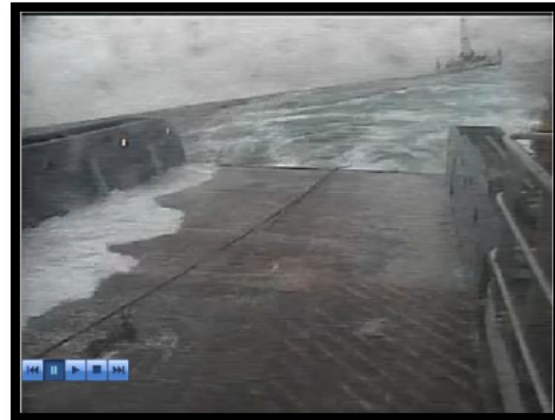
Figure 65: Port Forward CCTV stills showing fluctuations in towline tension. Still on left shows high tension at 10:54:48, demonstrated by the stiffness of the hogging chain (bottom right of still) and towline appearing to lead nearly horizontally toward KULLUK. Still on right shows low tension at 10:54:52, a mere 4 seconds later, with a slack Deadman chain and towline on the deck. (AIVIQ CCTV Provided by ECO)
