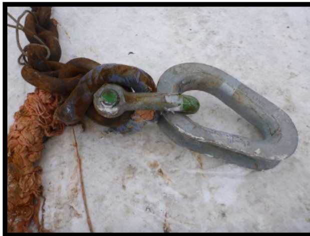
Figure 75: Photo of recovered emergency towline (eye on the KULLUK end of the emergency towline) showing missing thimble lashings allowing towline to separate from hard thimble. Blue Cordura® protection is also damaged. ( USCG Photo )
