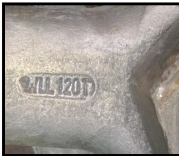
Figure 55: Photo of Working Load Limit Stamped on Bow of 120 Van Beest Green Pin® Super Shackle. (USCG Photo)
