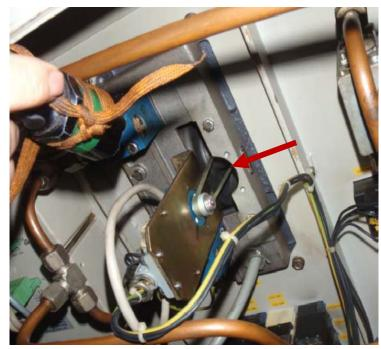
loosened, went unnoticed and caused flooding of the machinery space of an Offshore Supply vessel; A wire chafed and grounded out cutting power to critical combustion controls while a vessel was at the dock, but not long after transiting a narrow Caribbean harbor entrance.
