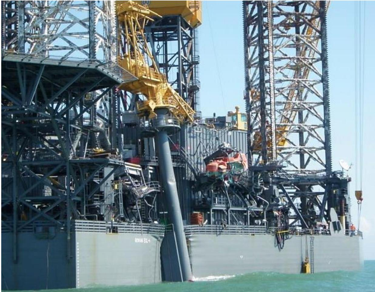
**The extensive damage to the port side of the *Rowan EXL I*, including its destroyed survival crafts (orange-colored) near the center of the photo. Photo provided by the Coast Guard.**
