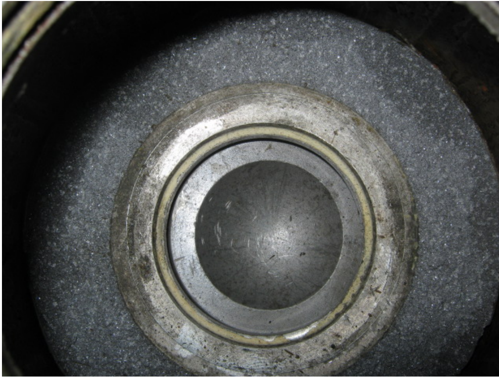
Figure 3.19: Close-up Photograph of Flapper Assembly Failure
