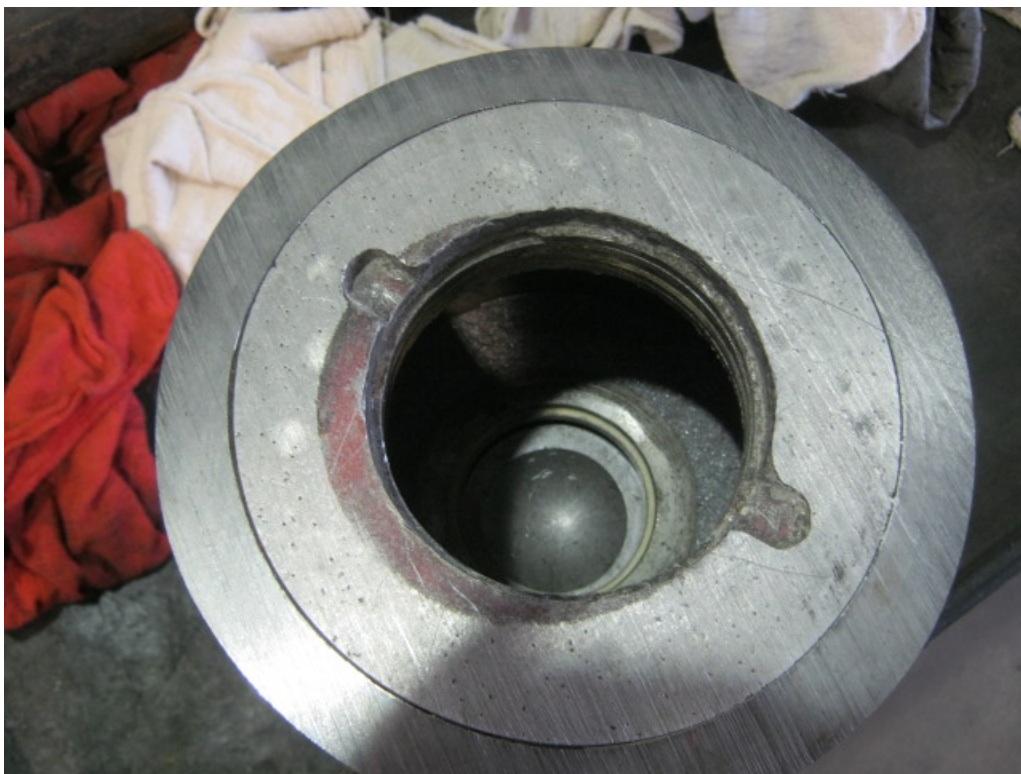
Figure 3.18: Photograph of Flapper Assembly Failure
