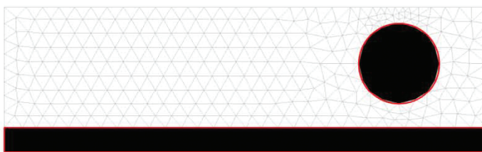
Figure 3 Non-rectangular geometry with an unstructured tetra-mesh
