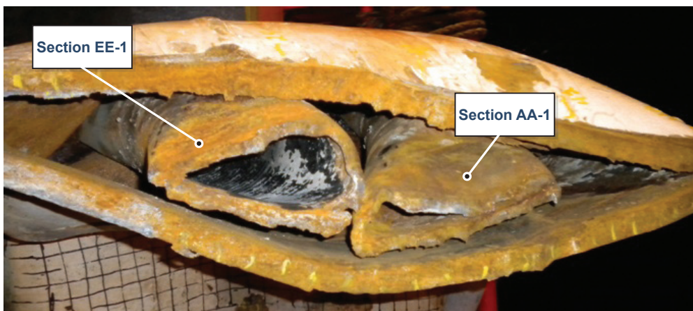
Figure 3 Sheared Section of the Recovered Riser at the Lower Kink End with the Drill Pipe Sections EE-1 and AA-1
