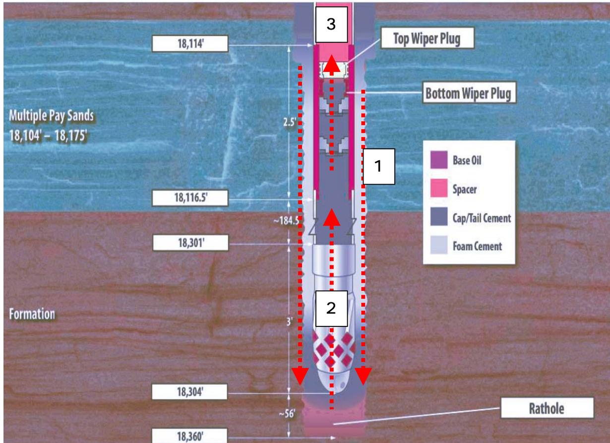
Figure 2.4 – Shoe Track hydrocarbon penetration paths.<sup>24</sup>
