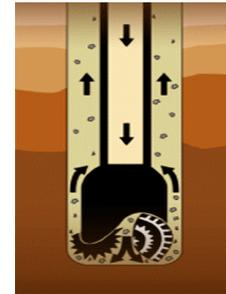
Cuttings in circulating drilling fluids.<sup>23</sup>
