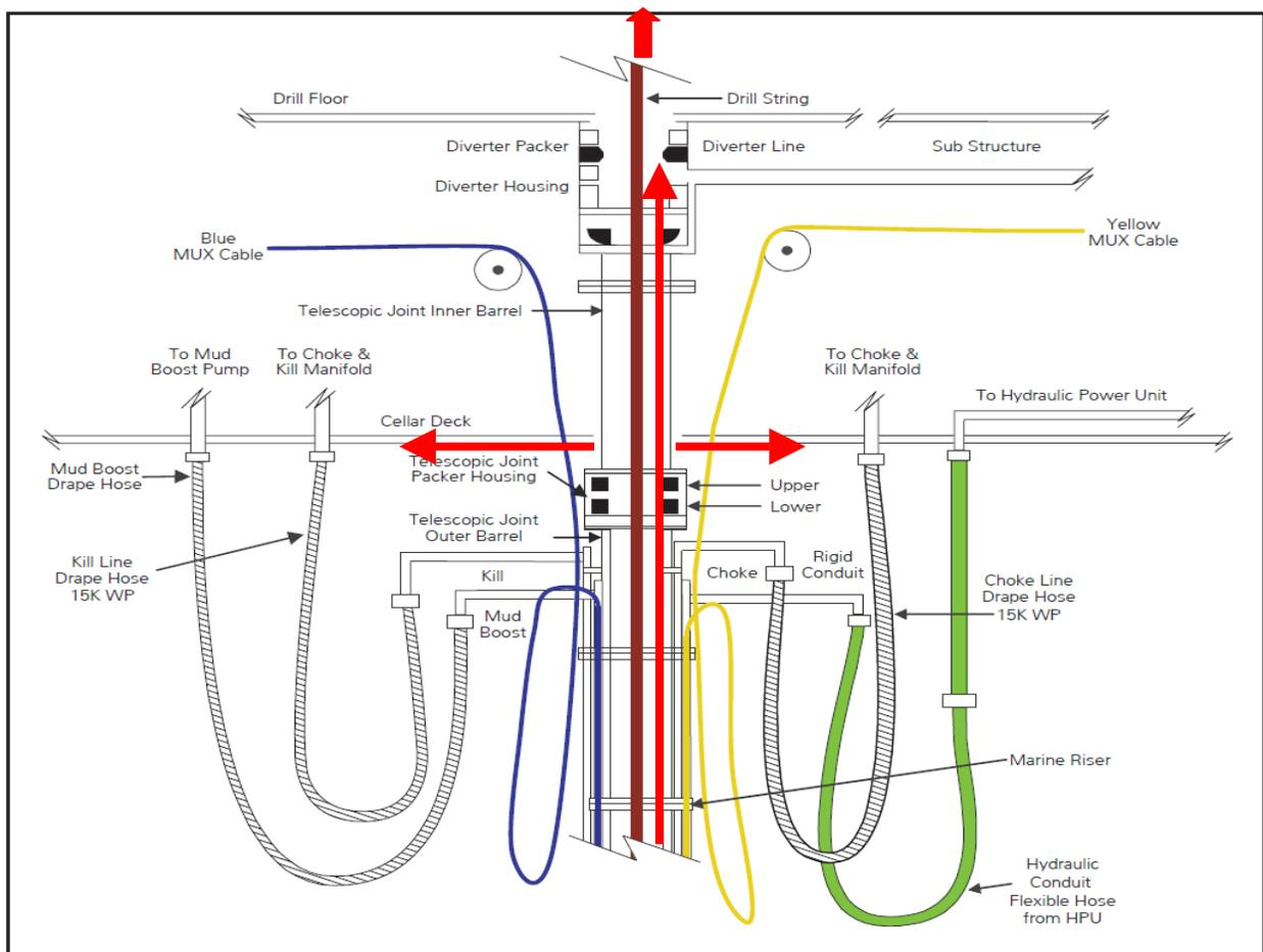
Figure 2.13 – Configuration of drilling riser, drill pipe, and other equipment in Moonpool area.<sup>44</sup>
