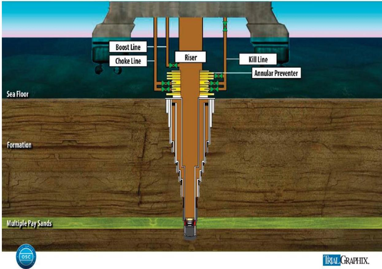
Figure 1.20 – Illustration of the "choke" and "kill" lines.<sup>86</sup>
