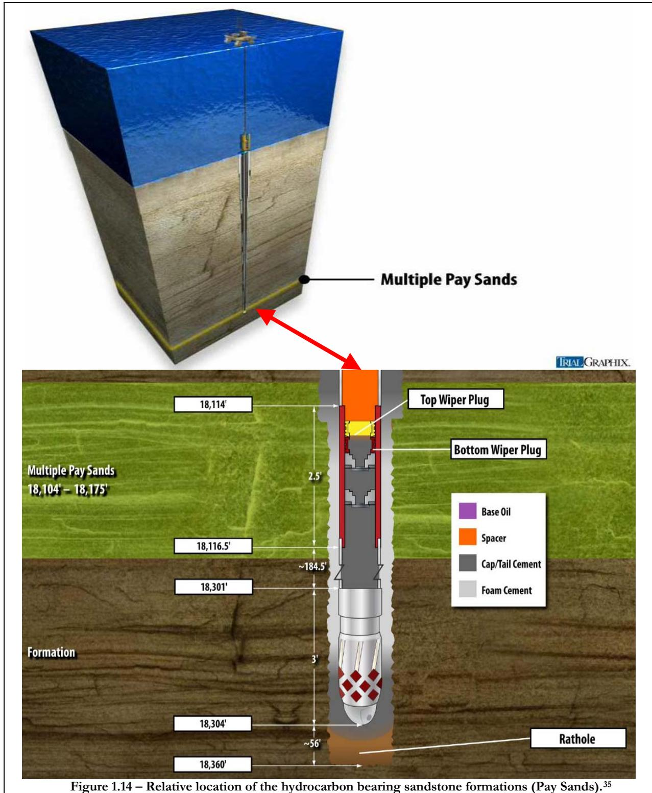
Figure 1.14 – Relative location of the hydrocarbon bearing sandstone formations (Pay Sands).<sup>35</sup>
