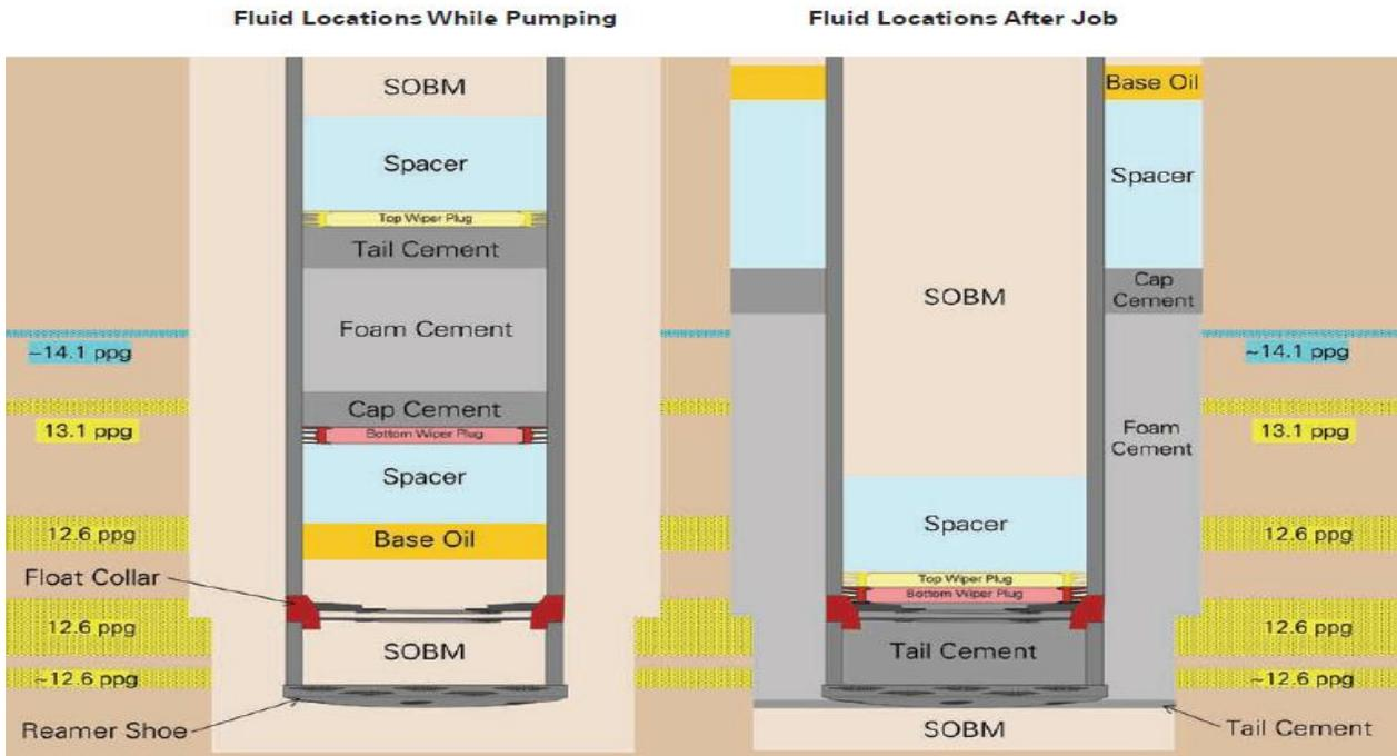
Figure 1.19 – Cement fluid locations.<sup>71</sup>
