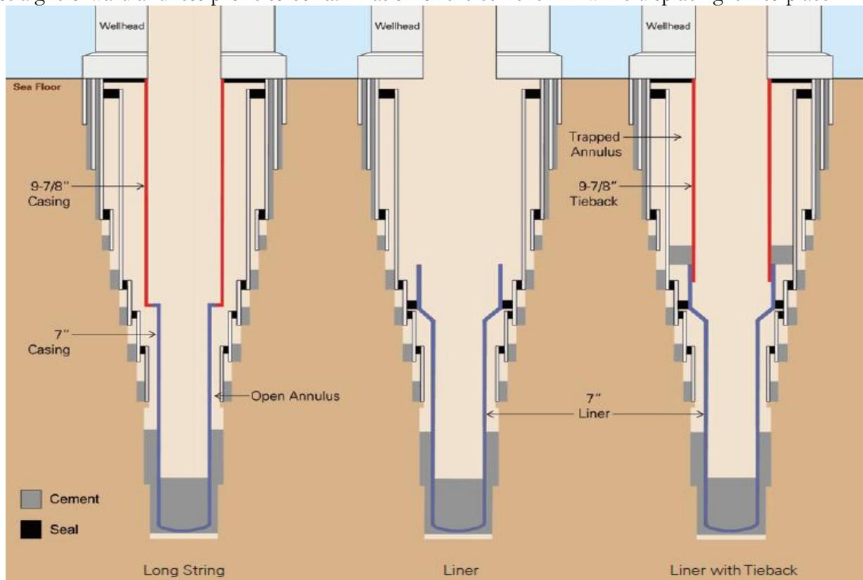
**Figure 1.15 – Long String, Liner and Liner with Tieback.<sup>48</sup>**
