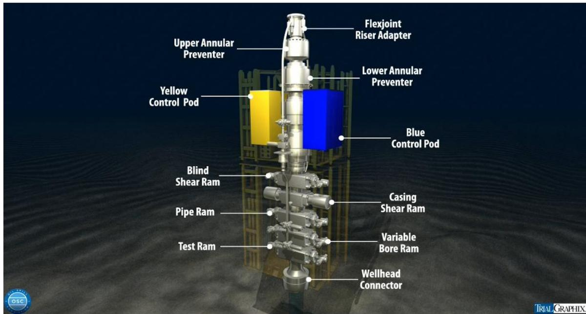
Figure 1.8 – BOP Assembly.<sup>27</sup>
