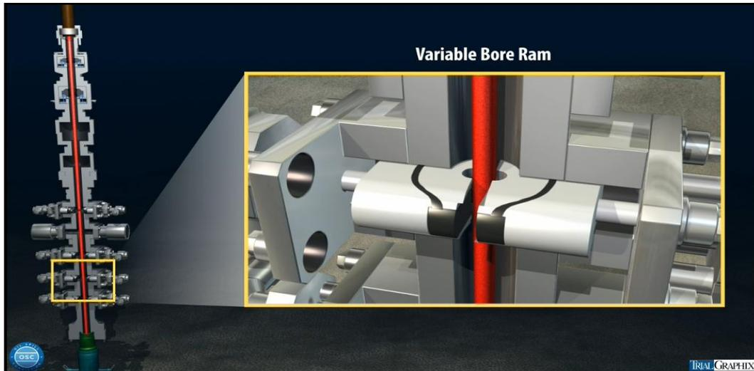
Figure 1.10 – Variable Bore Ram.<sup>28</sup>
