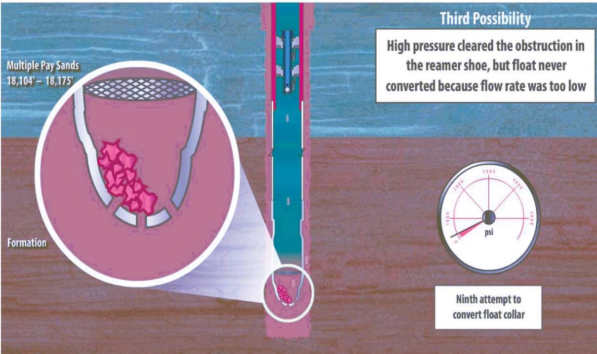
Figure 2.6 – Float collar conversion failure.<sup>26</sup>
