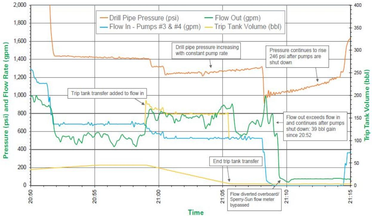
Figure 1.23 – Flow indication graph showing anomalies (real-time data).<sup>101</sup>
