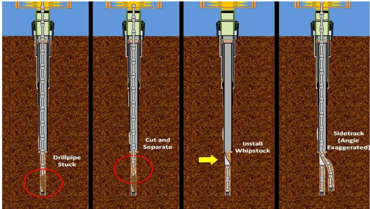
Figure 1.4 – Illustration of sidetrack procedures.<sup>19</sup>
