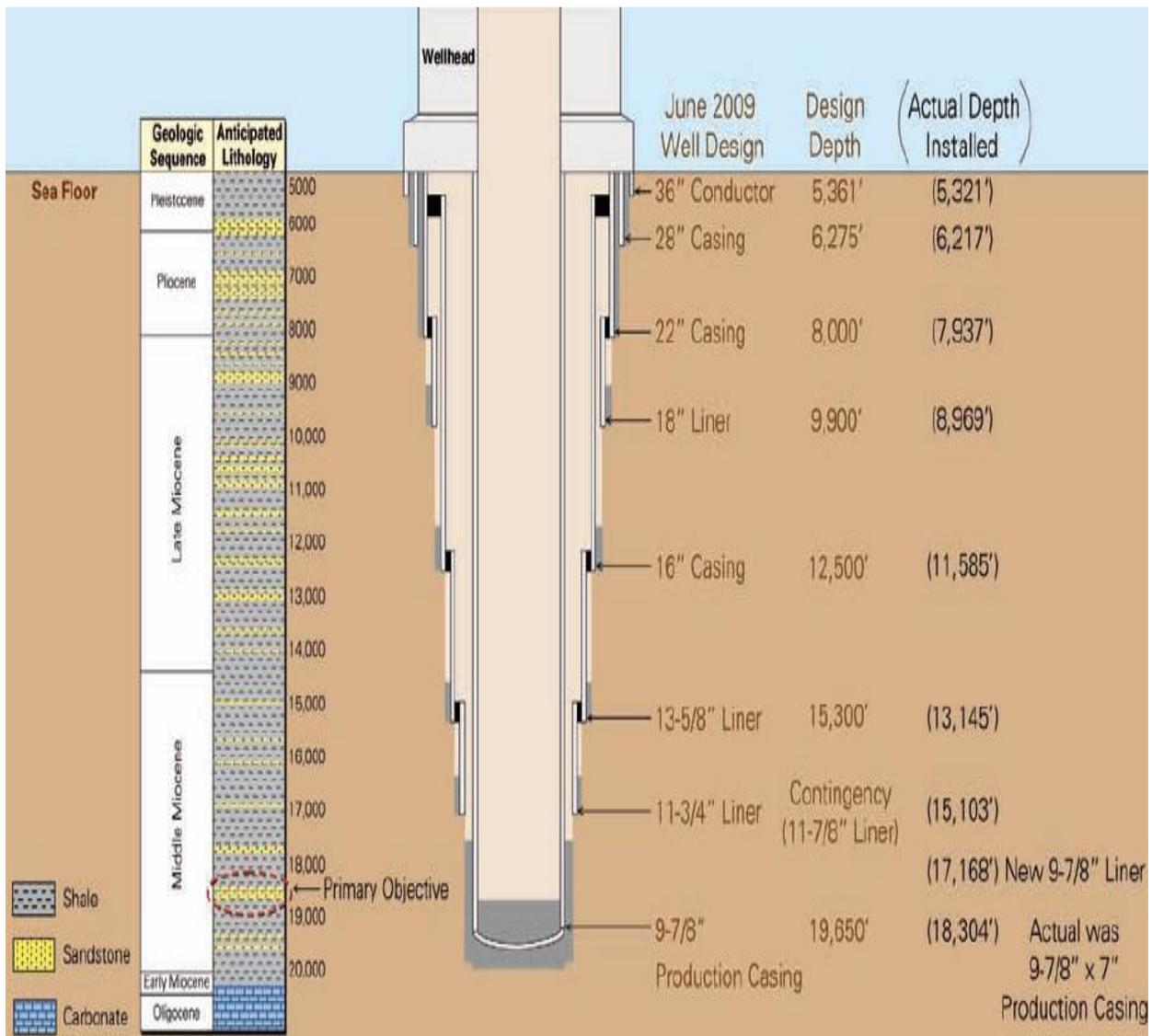
**Figure 1.3 – Geology, original well design and installed depth.<sup>12</sup>**
