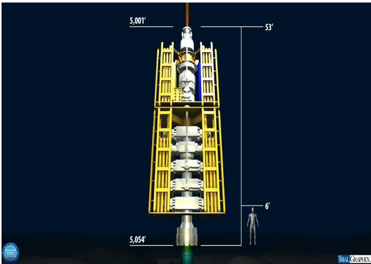
Figure 1.7 – Blowout Preventer (BOP).<sup>26</sup>
