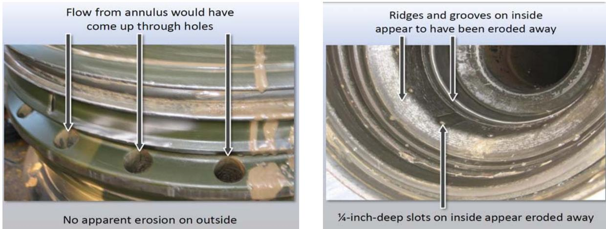
**Figure 2.3 – Photographs of exterior (left) and interior (right) of 9<sup>7</sup>/<sub>8</sub> in Hangar Seal Assembly.<sup>19</sup>**
