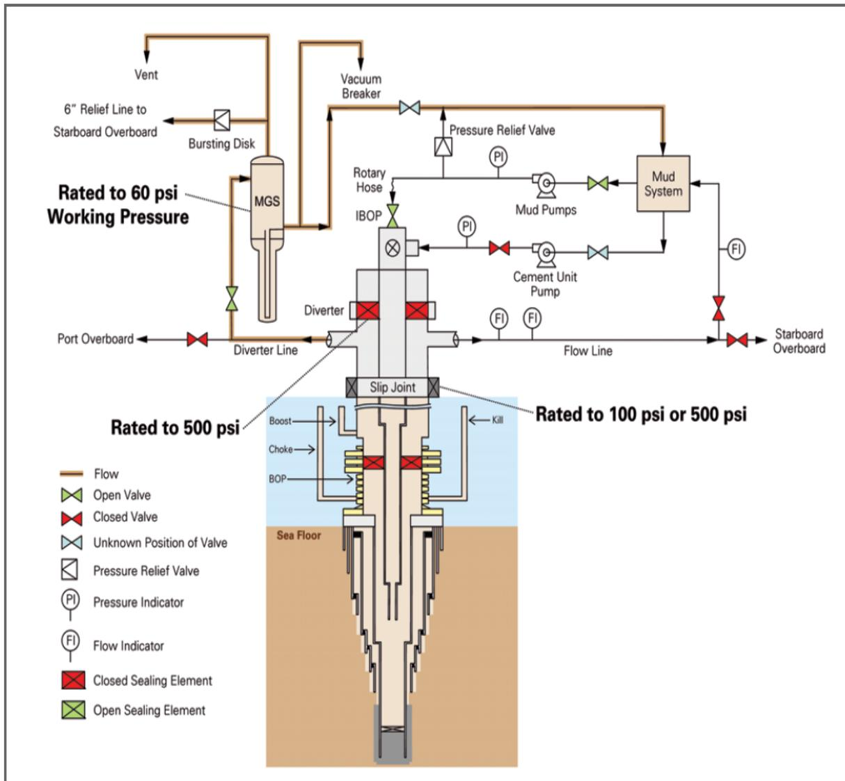
Figure 2.11 – Schematic of *Deepwater Horizon* surface equipment.<sup>39</sup>
