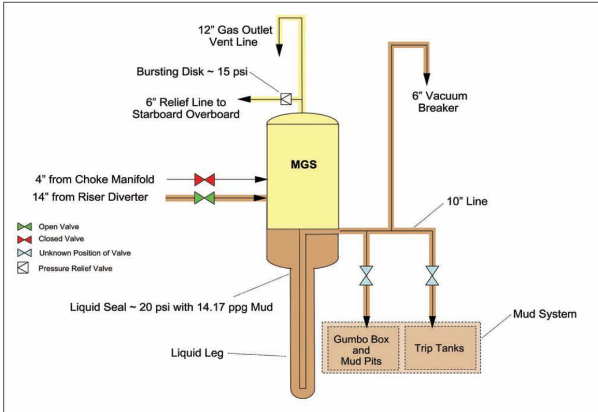
Figure 2.12 – Schematic of *Deepwater Horizon* Mud Gas Separator.<sup>40</sup>
