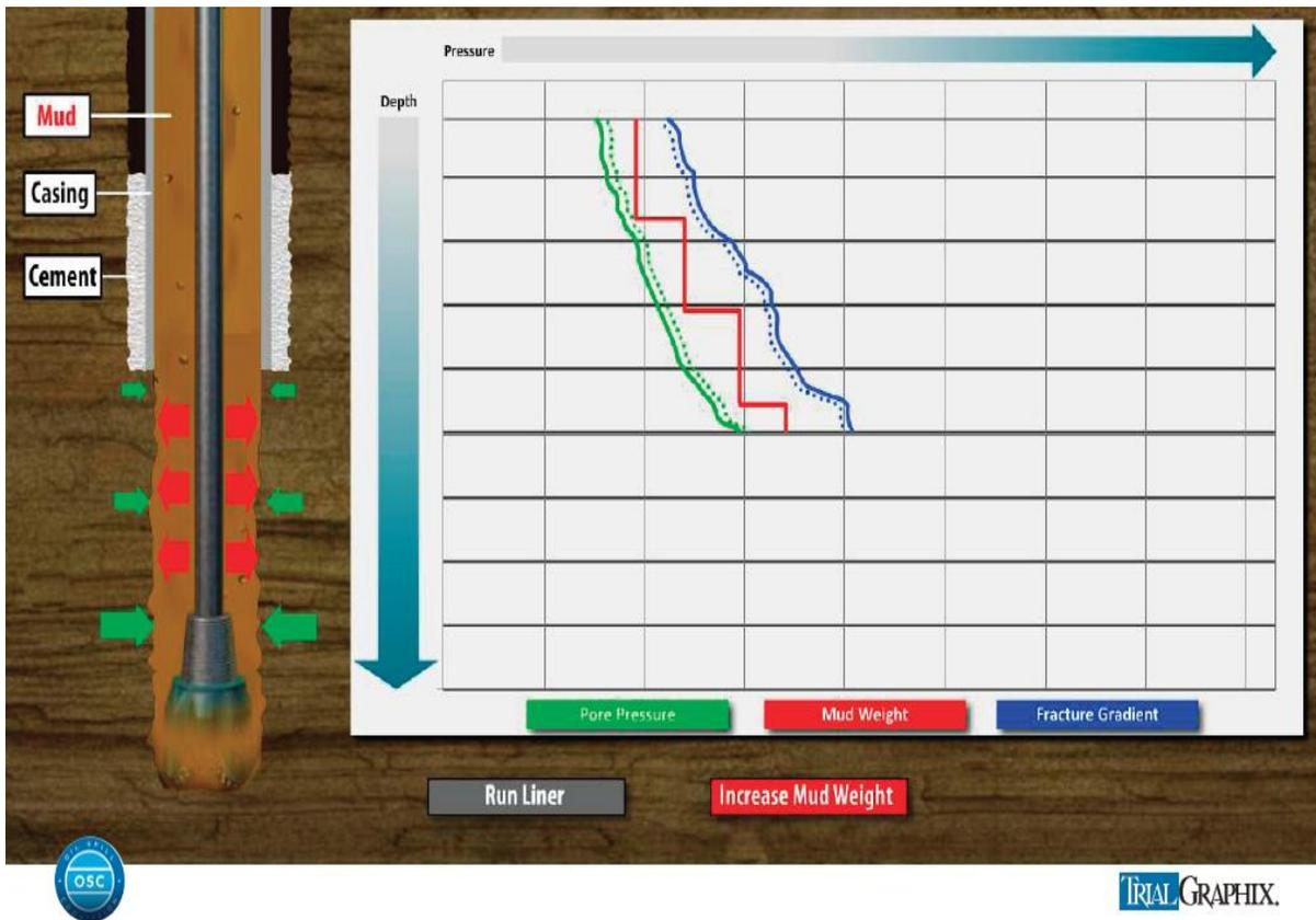
Figure 1.6 – Illustration of Borehole Pressures and the Drilling “Window”.<sup>24</sup>
