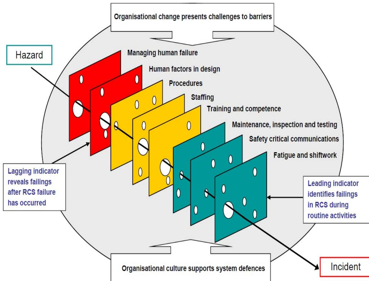
Figure 3.1 – Accident resulting from successful penetration of multiple defensive barriers.<sup>4</sup>
