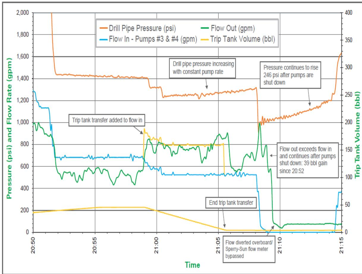
Figure 2.8 – Real-Time data (April 20, 2010) during last portion of mud transfer operations.<sup>35</sup>
