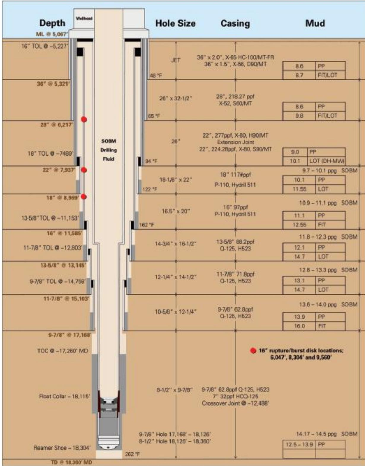
Figure 1.5– The Macondo actual well casing run.<sup>22</sup>
