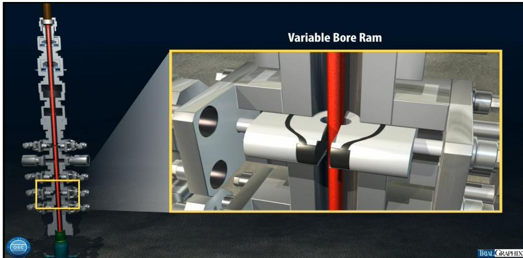
Figure 1.10 – Variable Bore Ram.<sup>28</sup>
