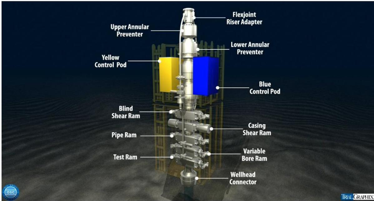
Figure 1.8 – BOP Assembly.<sup>27</sup>
