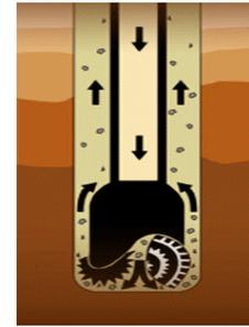
Cuttings in circulating drilling fluids.<sup>23</sup>
