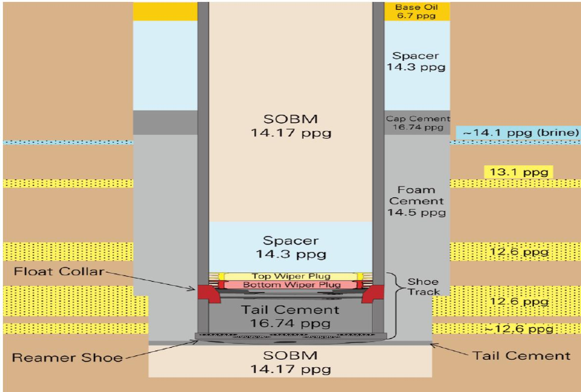
**Figure 2.5 – Planned cement placement.**<sup>25</sup>
