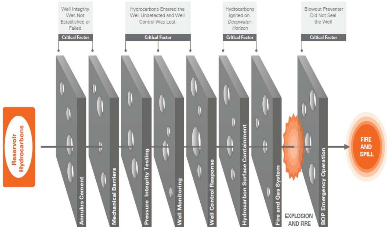
**Figure 3.2 – BP’s analysis of defensive barrier penetration leading to the Macondo blowout.<sup>7</sup>**
