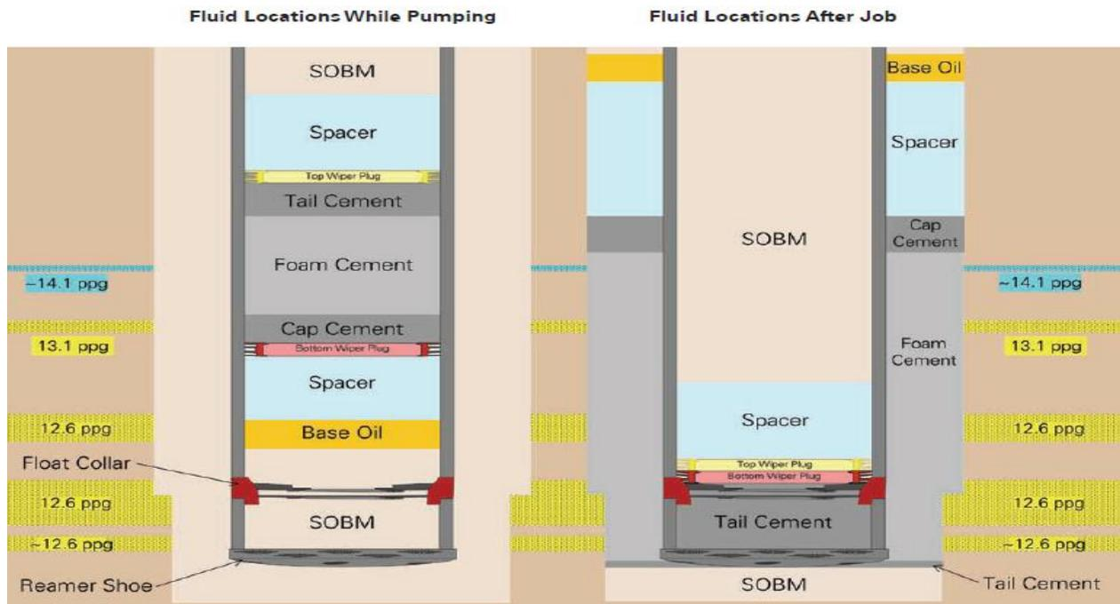
Figure 1.19 – Cement fluid locations.<sup>71</sup>
