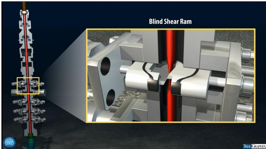
Figure 1.11 – Blind Shear Ram.<sup>28</sup>
