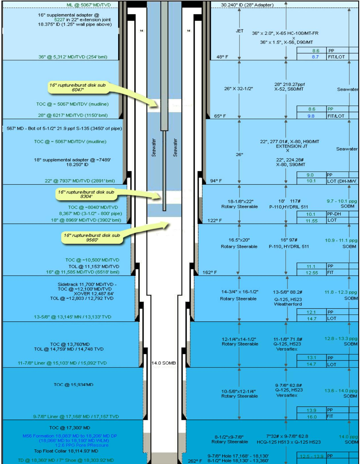
Figure 2.1 – Well schematic.
