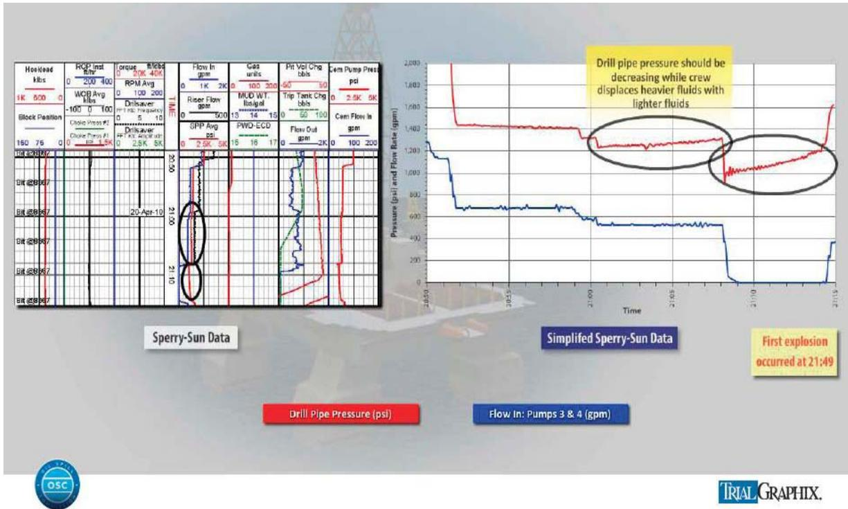
Figure 1.22 – Drill pipe pressure showing pressure increase.<sup>100</sup>
