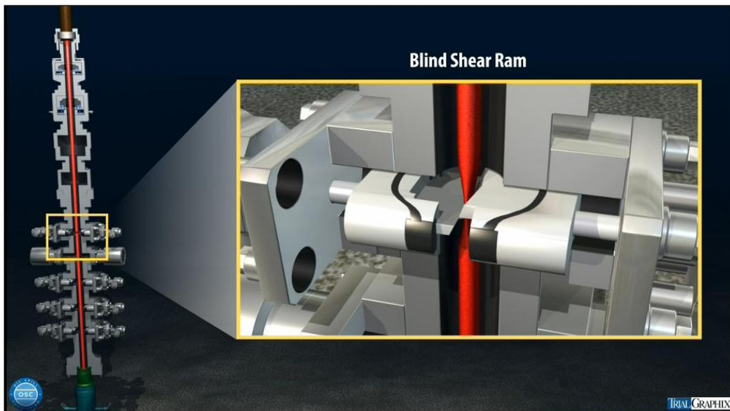
Figure 1.11 – Blind Shear Ram.<sup>28</sup>
