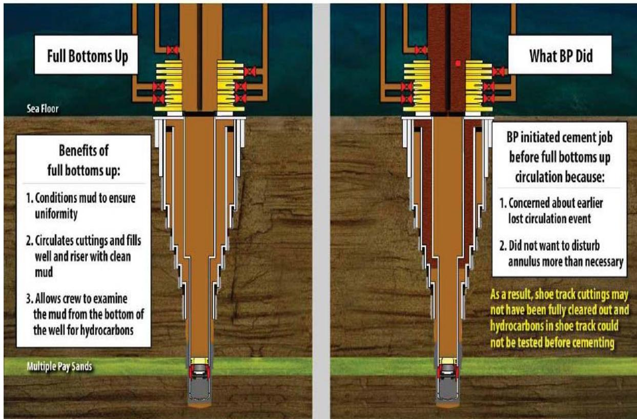
Figure 1.18 – Illustration of *bottoms up*.<sup>70</sup>
