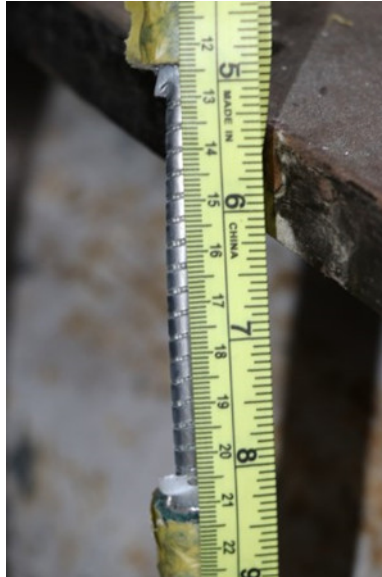
Figure 35: Conduit separation after cycling the release handle with a broken cable conduit/liner. Credit: CG.
