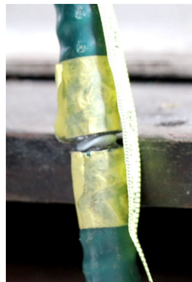
Figure 25: Compression of PTFE liner during the third open cycle of the release handle (outer conduit layers are now nearly touching). Credit: CG.
