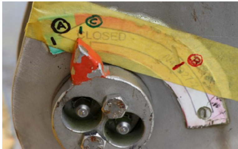
Figure 16: Locking Shaft Positions: A = maximum closed position (against the stop), B = Open (no load applied), and C = as found closed position for Auger Lifeboat 6. Credit: CG.
