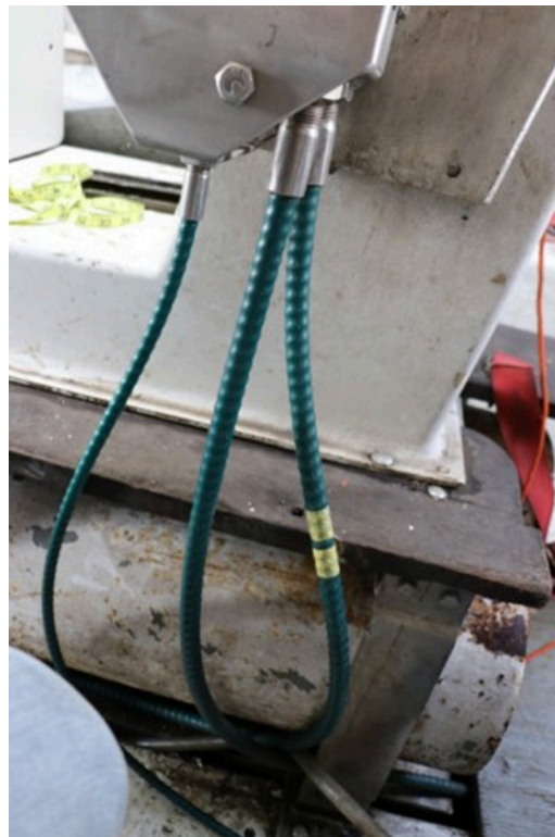
Figure 17: Aft hook control cable marked for simulated damage. Credit: CG.
