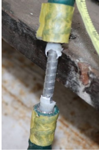
Figure 31: Broken polyethylene liner. Credit: CG.
