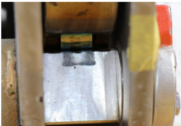
Figure 33: Locking shaft (cam) position upon breakage of the polyethylene liner and separation of the cable conduit. Credit: CG.
