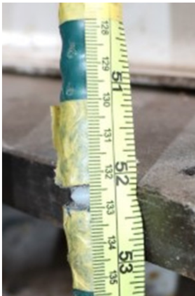
Figure 23: Compression of PTFE liner during the first open cycle of the release handle (outer conduit separation reduced to 6 mm). Credit: CG.
