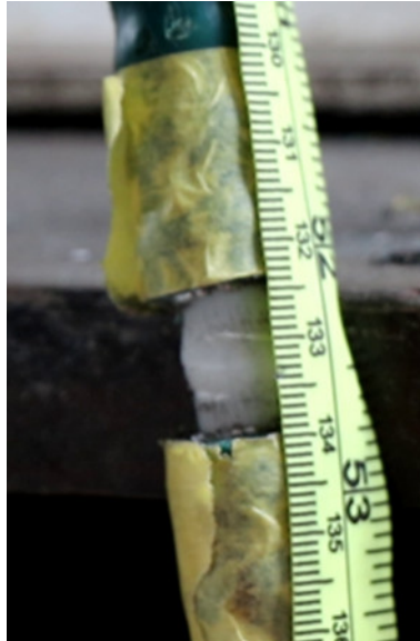
Figure 27: Translucent lines near the base of the compressed area of the polyethylene liner (after 12 cycles; started at 5 cycles). Credit: CG.
