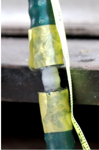
Figure 26: Maximum separation of the outer conduit layers and corresponding polyethylene stretch during the third close cycle of the release handle. Credit: CG.
