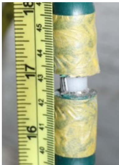
Figure 21: Measurement prior to removing the last few steel strands (9 mm). Credit: CG.
