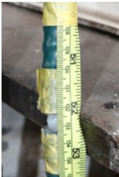
Figure 24: Distortion of PTFE liner after the first open/close cycle of the release handle (outer conduit separation increased to 12 mm). Credit: CG.
