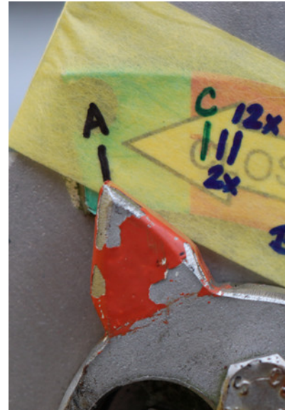
Figure 28: Locking shaft positions observed: A = maximum closed position C = as found closed position for Auger LB6 2x = movement toward open after 2 cycles, 12x = movement toward open after 12 cycles; locking shaft is shown in the closed position (picture taken after testing). Credit: CG.
