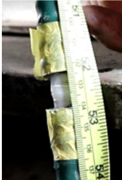
Figure 29: Separation after two activation cycles with the first cut in the polyethylene liner (increased by 1 mm). Credit: CG.
