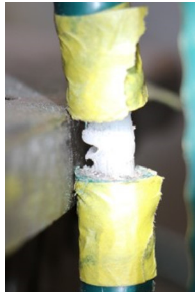
Figure 30: Distortion of the cut area (first cut) after two activation cycles. Credit: CG.
