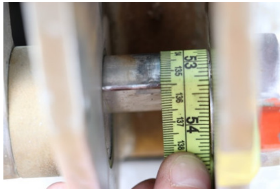
Figure 14: Measuring from locking shaft opening (notch) fillet/radius (looking down from the front side of the hook). Credit: CG.
