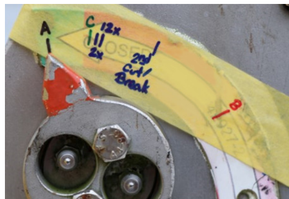
Figure 34: Locking shaft positions observed – the "break" observed in Step 11 put the locking shaft approx. halfway between closed ("C") and open ("B"); locking shaft is shown in the closed position. Credit: CG.
