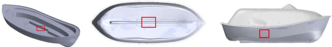
Figure 22: Sampling locations for fractographic analysis. Credit: DNV-GL.
