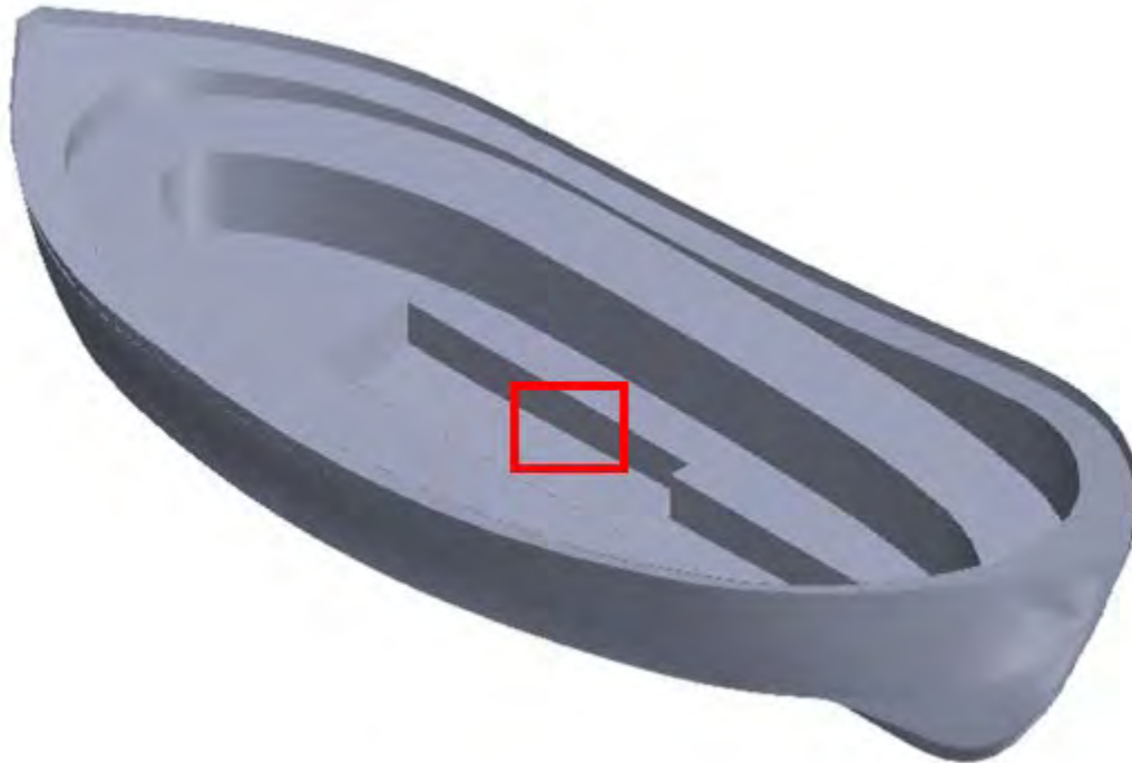
Figure 44. 3D representation of the approximate location of Sample C-1. The crack observed was located at the interior of boat at the fiberglass-engine mount interface.
