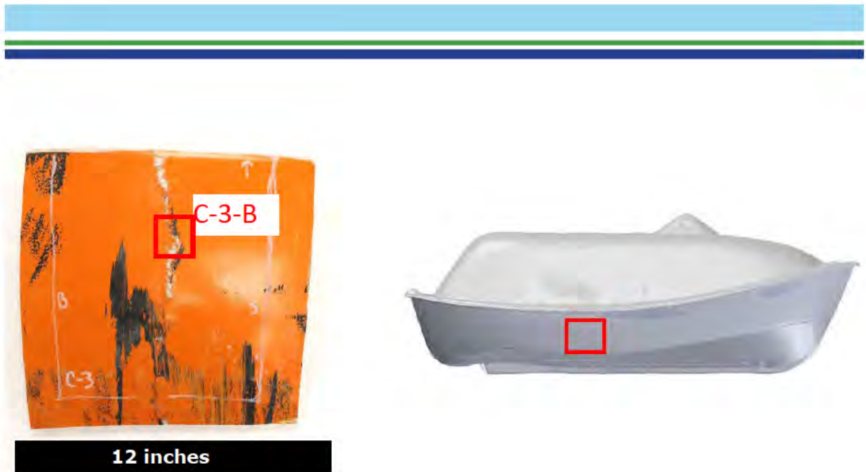
Figure 173. Photograph of Sample C-3 and schematic showing the location where the sample was removed from the outer hull. Sample C-3 was located 11.4 feet from the aft of Lifeboat 6. The location of the sample examined in the SEM, Sample C-3-B, is shown. Ruler are in inches.
