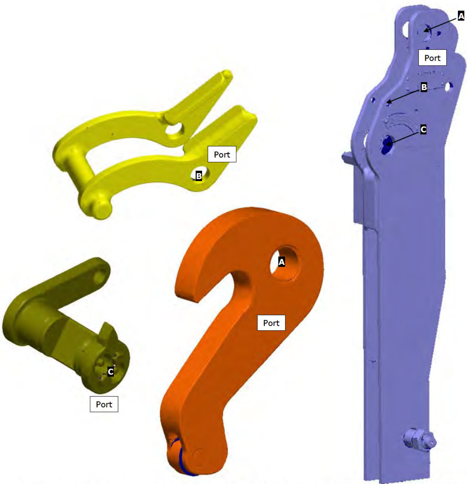
Figure 77. Laser scans of Subject Aft Hook components displayed individually. From left to right: the locking shaft (gold), the keeper (yellow), the hook (orange), and the housing (purple). The Locations A, B, and C correlate to the centerlines of the components and their respective positions in the housing.
