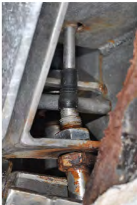
Figure 28. Photograph of the Subject Release Unit showing the as-found condition of the bulkhead nuts attaching the Subject Hydrostatic Cable to the Subject Release Unit.
