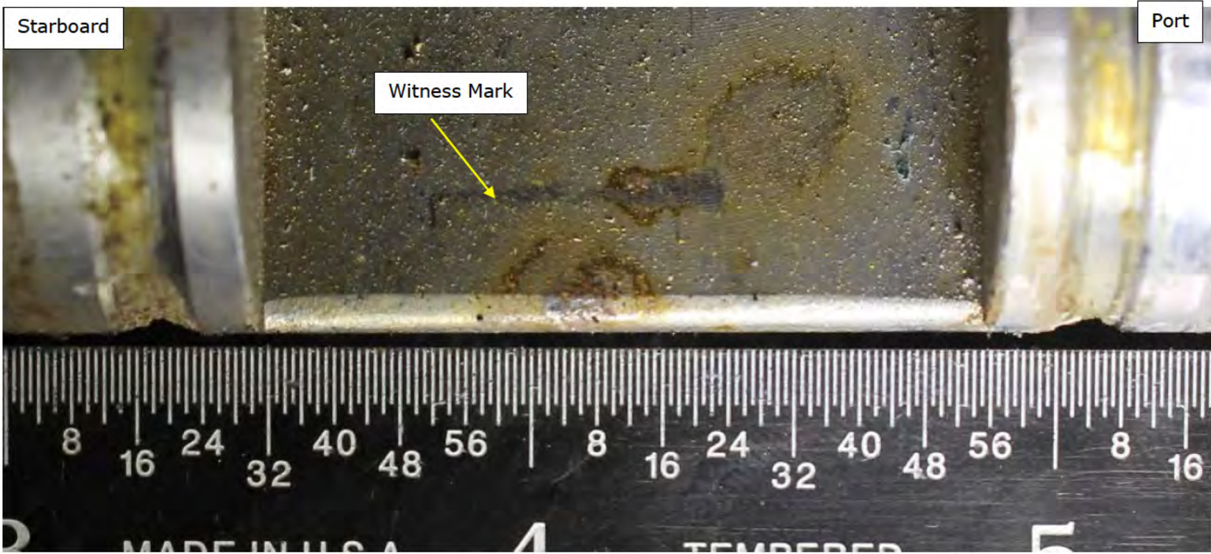
Figure 74. Photograph of the locking shaft from the Subject Forward Hook showing the edge between the round and flat of the locking shaft; area shown in Figure 73. Ruler is in inches.
