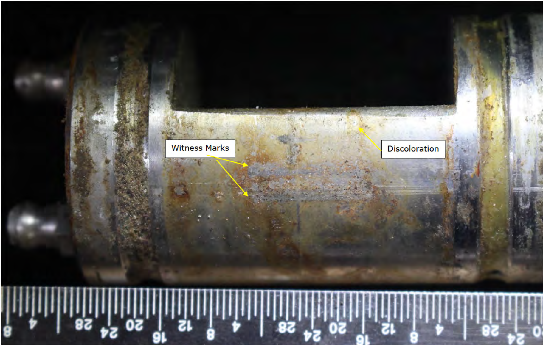
Figure 75. Photograph of the locking shaft from the Subject Forward Hook showing an area with corrosion attack on the round of the locking shaft; area shown in Figure 73. Ruler is in inches.
