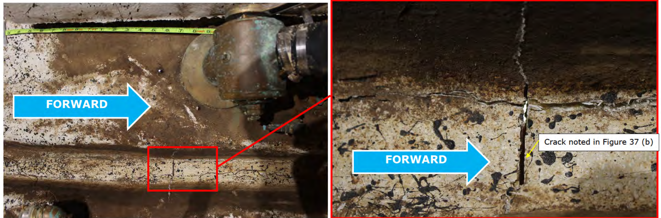
Figure 42. Photographs showing a transverse crack in the keel of the hull interior located 7.6 feet from the reference location. Tape measure is in feet.
