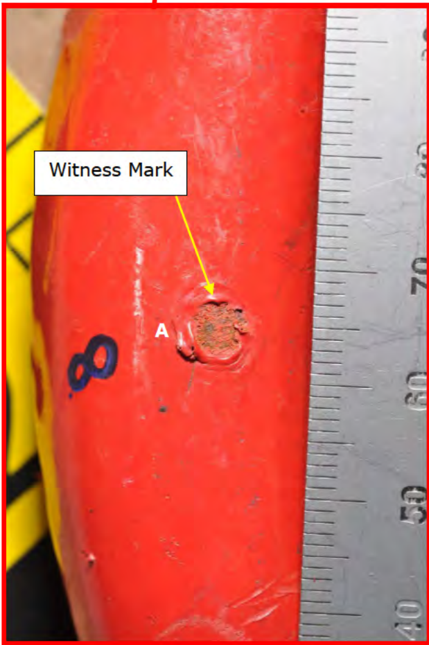
Figure 90. Photographs showing the Subject Aft Ring and locations where witness marks were identified. Ruler in top image is in inches and the ruler in the bottom image is in mm.
