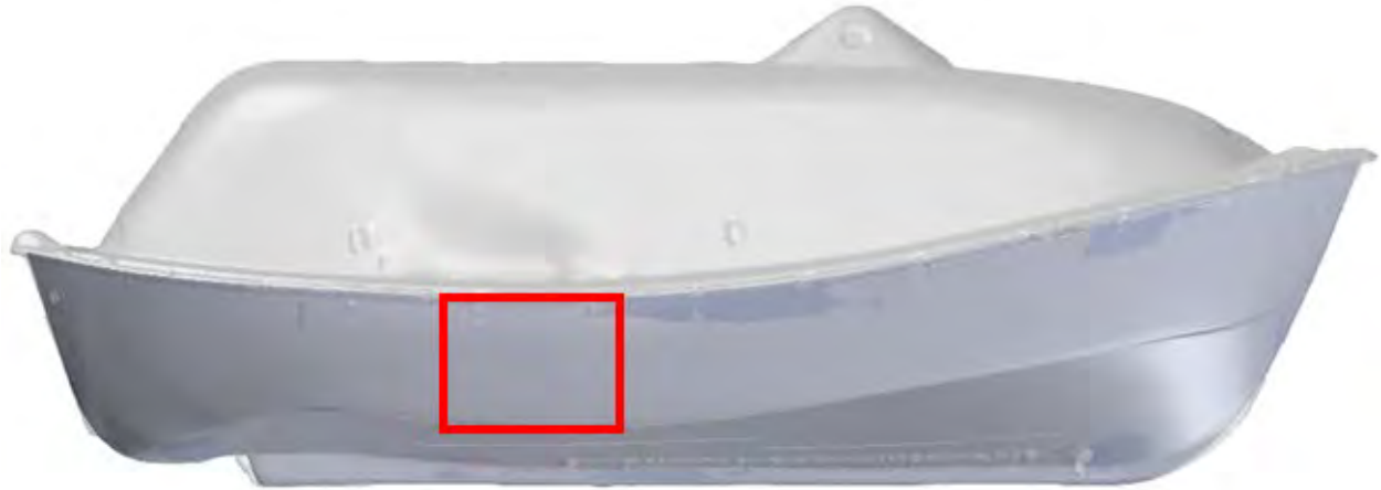
Figure 46. 3D representation of the approximate location of Sample C-3. The crack observed was located at the exterior of the hull on the starboard side. The crack ran from the hull-canopy interface towards the keel.
