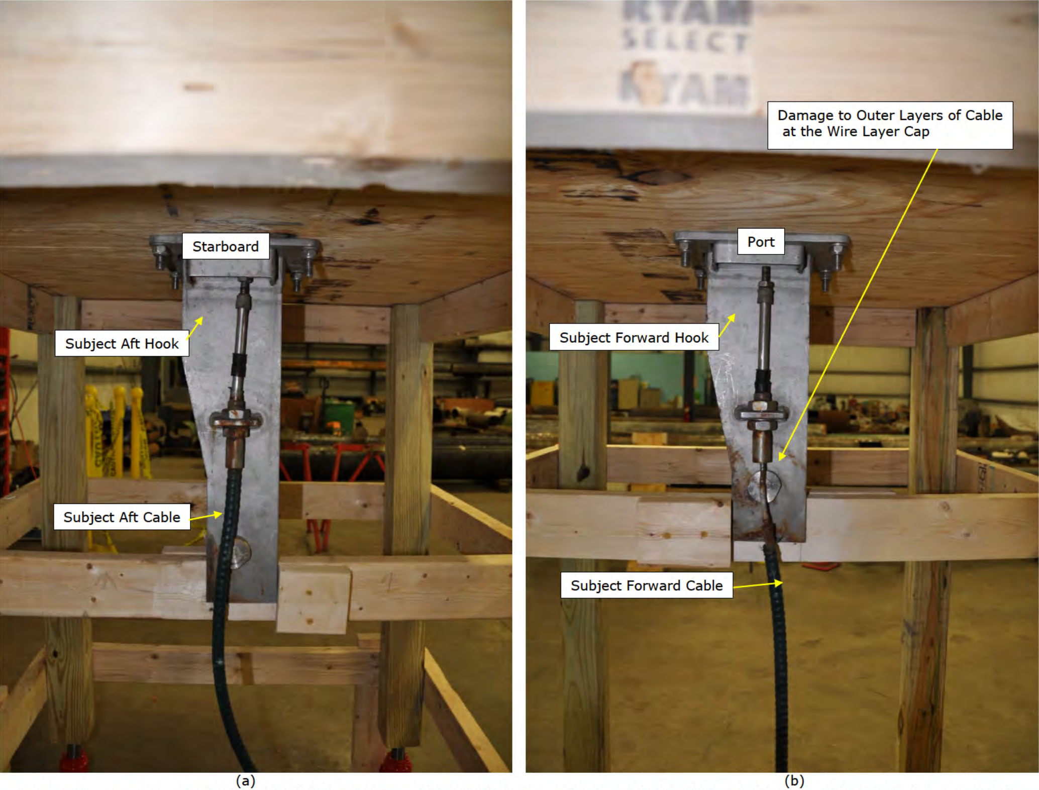
Figure 102. Photographs showing (a) Subject Aft Cable and (b) Subject Forward Cable at the Subject Aft and Subject Forward Hooks, respectively.
