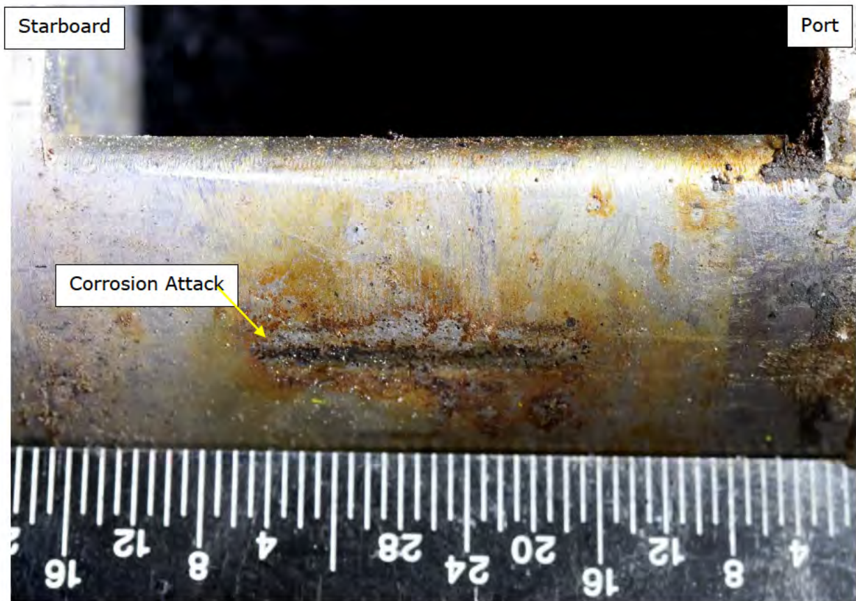
Figure 63. Photograph of the locking shaft from the Subject Aft Hook showing an area with corrosion attack on the round of the locking shaft. Ruler is in inches.
