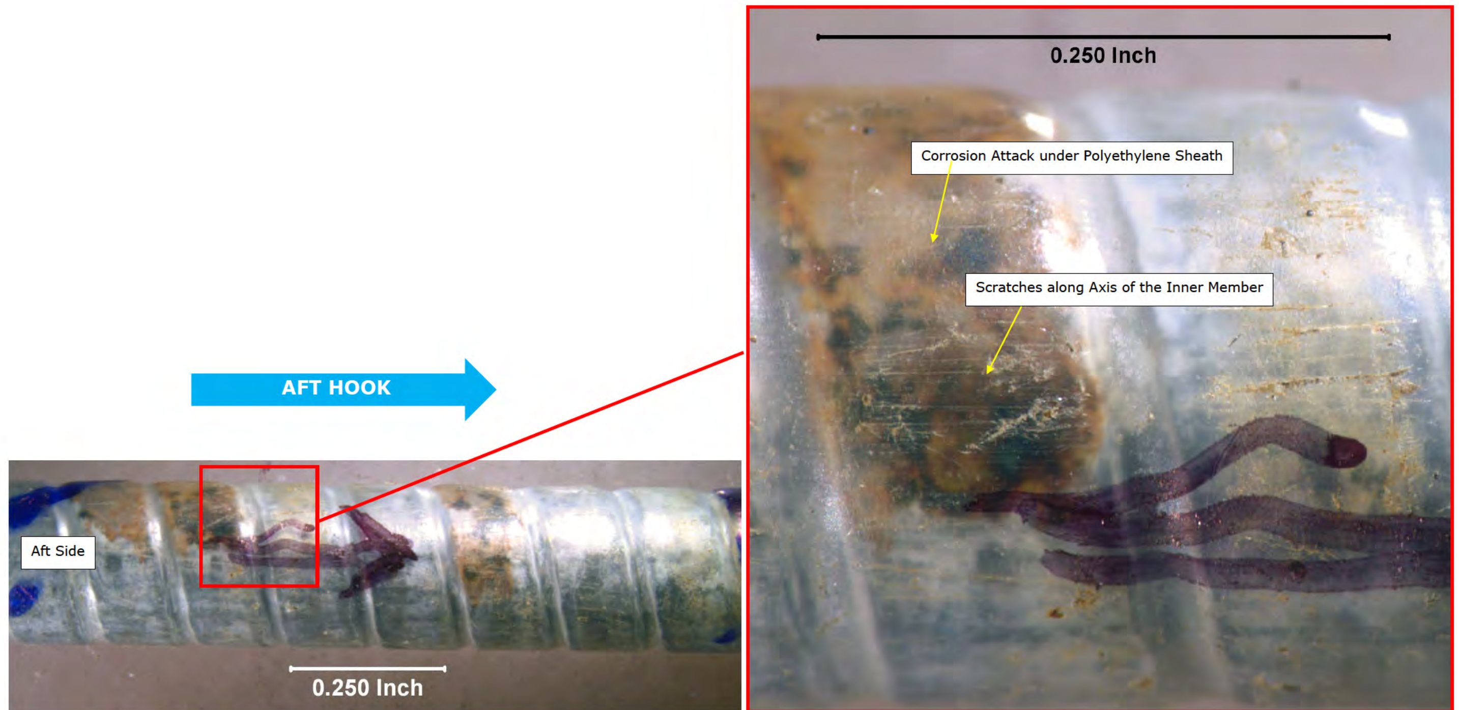
Figure 141. Light micrographs of the inner member of the Subject Aft Cable showing the detail of the minor corrosion attack to the binder wire and damage to the sheath layer of the inner member. The direction of the Subject Aft Hook is noted with the blue arrow.
