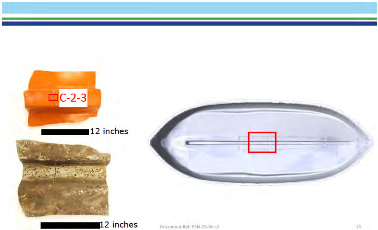
Figure 171. Photographs of Sample C-2 and schematic showing the location where the sample was removed from the inner hull. Sample C-2 was located near a crack in the keel. The location of the sample examined in the SEM, Sample C-2-3, is shown.
