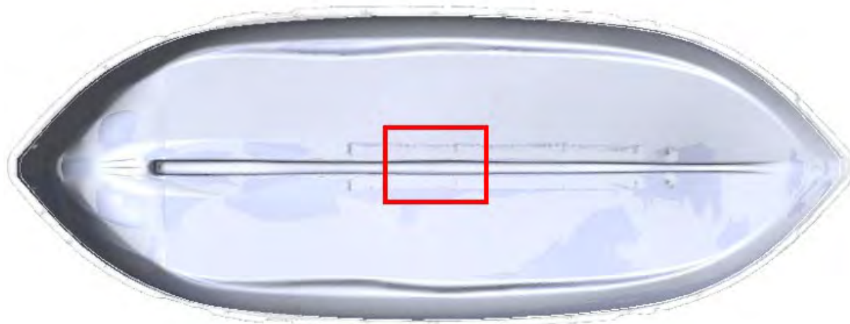
Figure 45. 3D representation of the approximate location of Sample C-2. The crack observed was located at the exterior of the hull on the keel of the boat. The crack propagated through the thickness of the keel.
