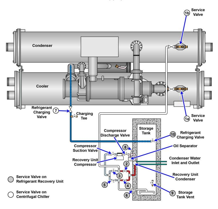
Adapted for testing purposes only from CARRIER, 19XRT Hermetic Centrifugal Liquid Chillers
