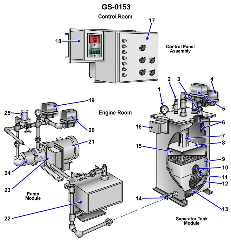
Adapted for testing purposes only from Operator, Unit and Direct Support Maintenance Manual Including Repair Parts and Special Tools List for Oil Water Separator
