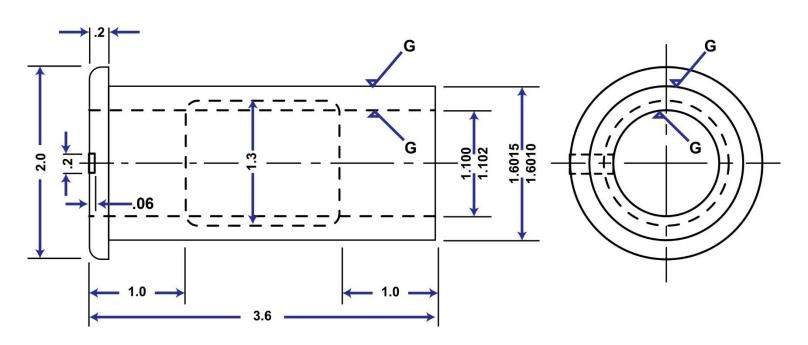
Bushing AISI 1095 SAE Carbon Steel Hardened and Tempered Designated Surfaces Ground To Specified Tolerances
