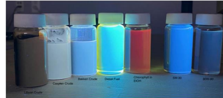
Figure 2: Fluorescence of a variety of oil samples. Also present is a chlorophyll sample.
