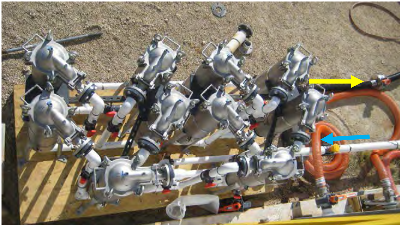
Figure 9. Plan view of the prototype filter skid at NRLKW. Blue arrow shows water entering the filter skid; yellow arrow shows water exiting the skid.
