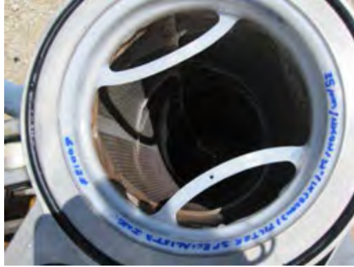
Figure 8. Nylon monofilament mesh filter bag secured in an Eaton Topline™ filter housing.
