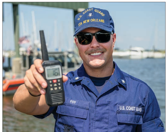
Coast Guard Petty Officer 3rd Class Charles Foy displays a handheld VHF radio in New Orleans on September 11, 2025. VHF-DSC, or very-high frequency-digital selective calling, radios are key to communicating on the water, allowing boaters to coordinate traffic patterns and reach out for help if they are in distress. Coast Guard photo by Petty Officer 3rd Class Anthony Randisi
