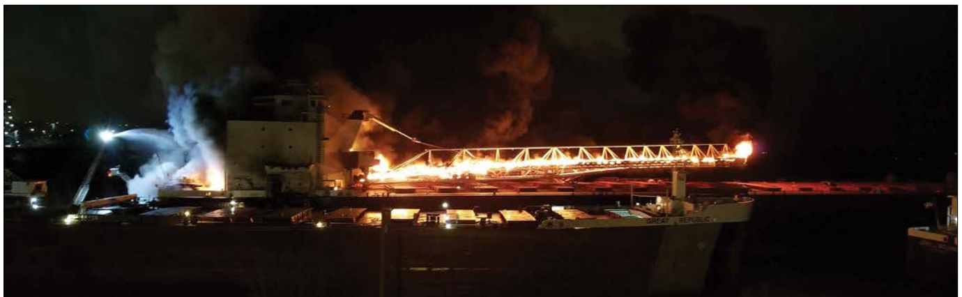
In February 2019, during winter layup in Toledo, Ohio, the St. Clair experienced a fire that rendered the ship a total constructive loss. Ice-clogged dockside hydrants and a frozen Lake Erie hampered fire suppression efforts. Coast Guard photo
