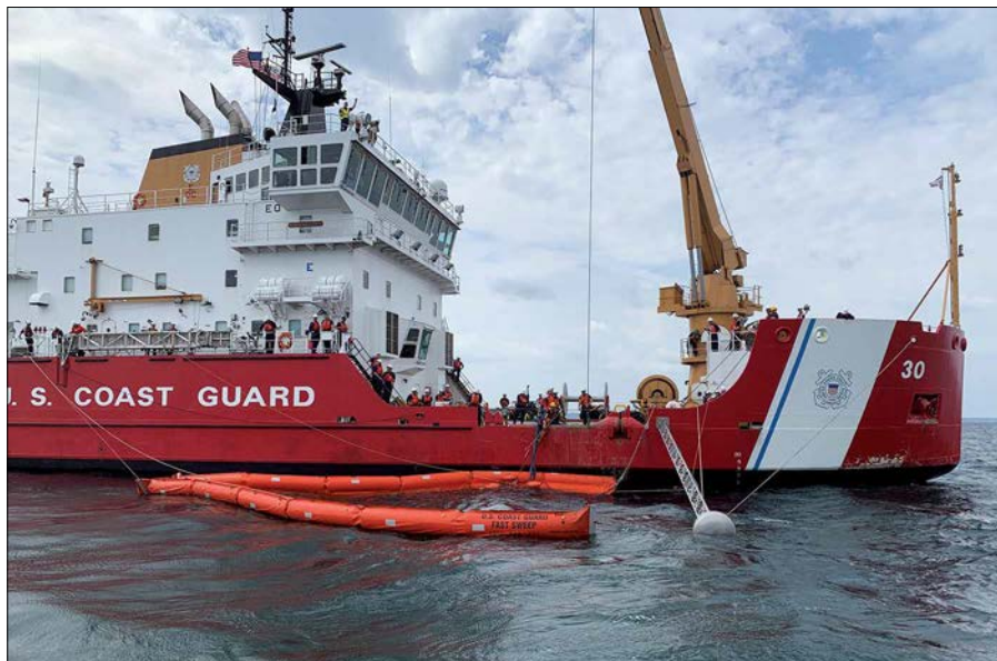
A U.S. Navy Supervisor of Salvage Vessel of Opportunity Skimming System is deployed from the Coast Guard Cutter Mackinaw on Lake Erie in 2021. Photo by Jerome A. Popiel
