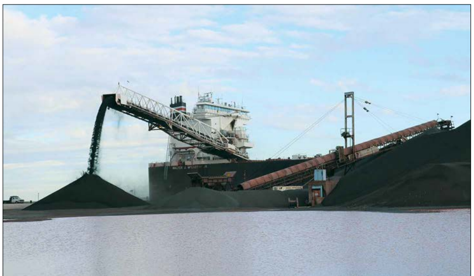
A Great Lakes freighter uses a self-unloading system at a Great Lakes port. The largest vessels plying the Great Lakes have the ability to self-unload with a conveyor belt system and a boom reaching up to 280 feet. This allows the discharge of cargo at virtually any dock in eight hours or less. Photo courtesy of Interlake Steamship Company
