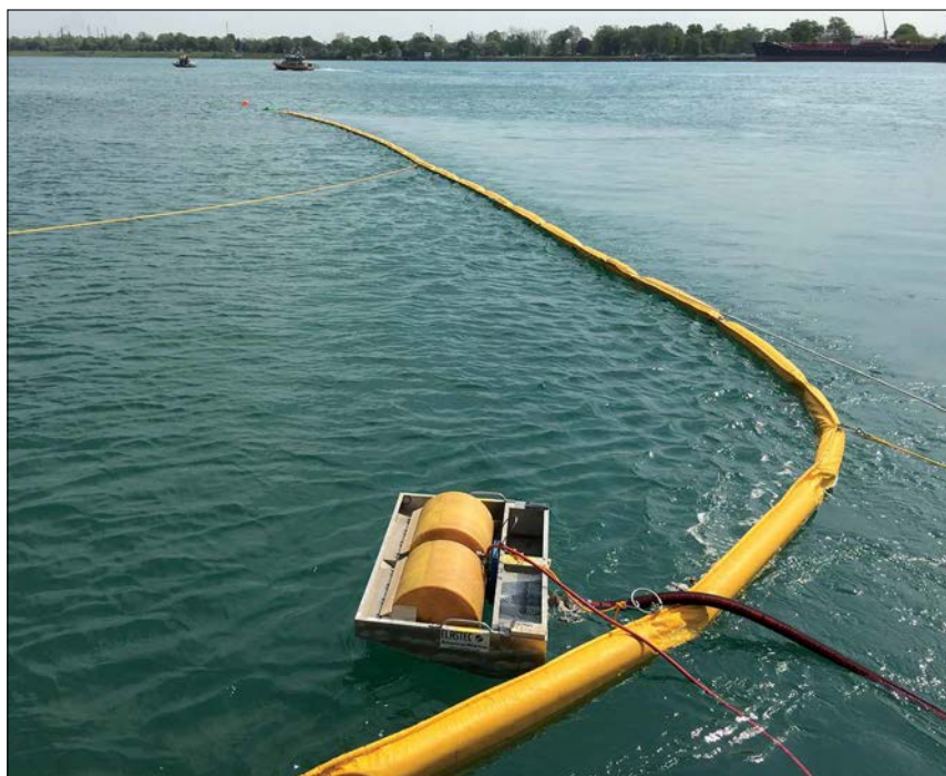
Containment boom is deployment on the St. Clair River during a 2017 joint U.S.-Canadian exercise. The international border essentially runs down the middle of the river in this photo. Photo courtesy of Jerome A. Popiel
