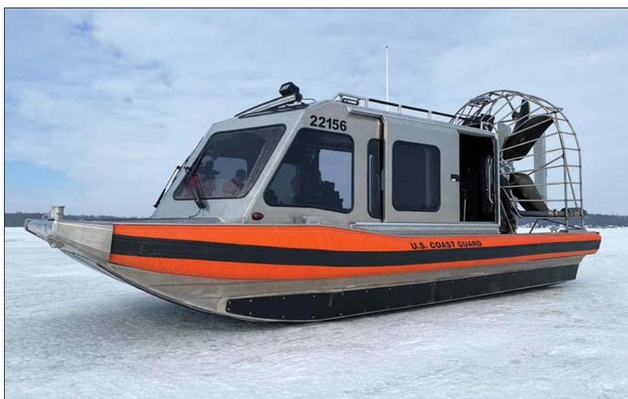
The CG-22156, a Special Purpose Craft-Ice Rescue Transport, deploys on the ice in Lake Erie. Units across the Great Lakes received 10 new special purpose crafts designed specifically for ice rescue transport up to 10 miles offshore. Coast Guard photo
