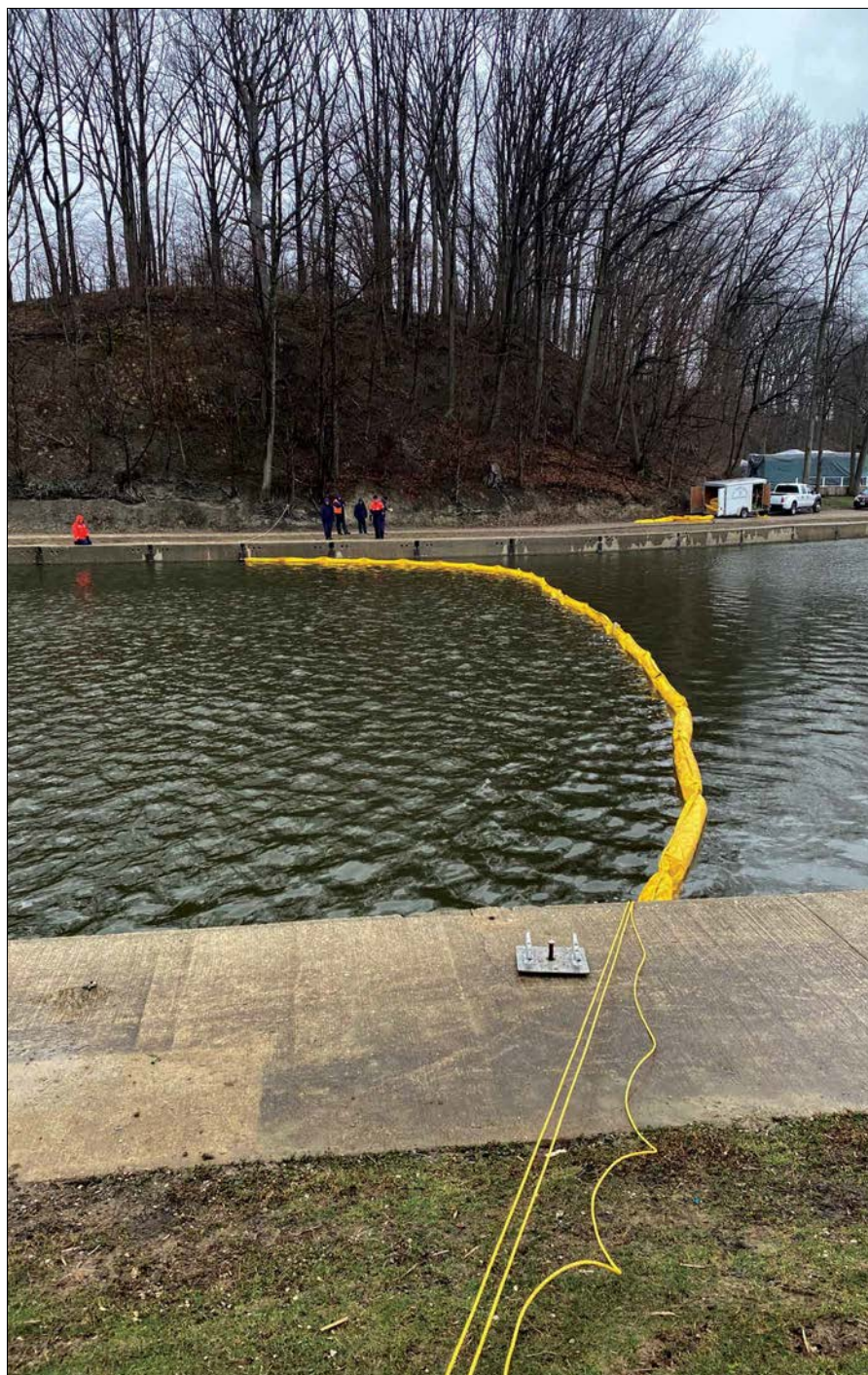
Containment boom is deployed across the Ashtabula River east of Cleveland, as part of the Rogue IV exercise held in April 2022. Coast Guard photo by Petty Officer 2nd Class Emily Duffy
