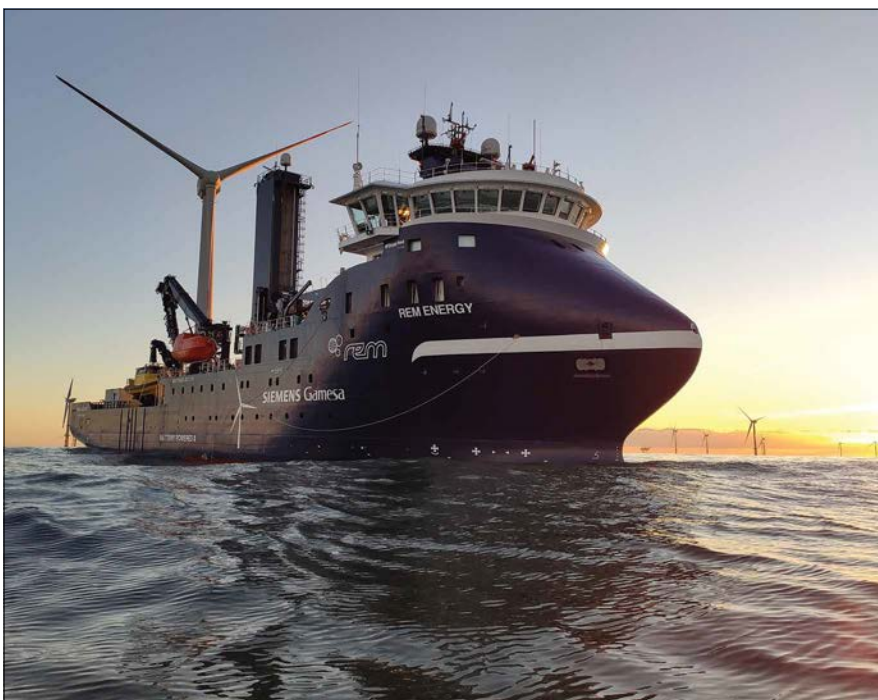
Siemens Gamesa-commissioned REM Energy , a new hydrogen-ready service operation vessel, is technically ready to operate emission free thanks to fuel cells and battery technology. Photo courtesy of REM Offshore AS
