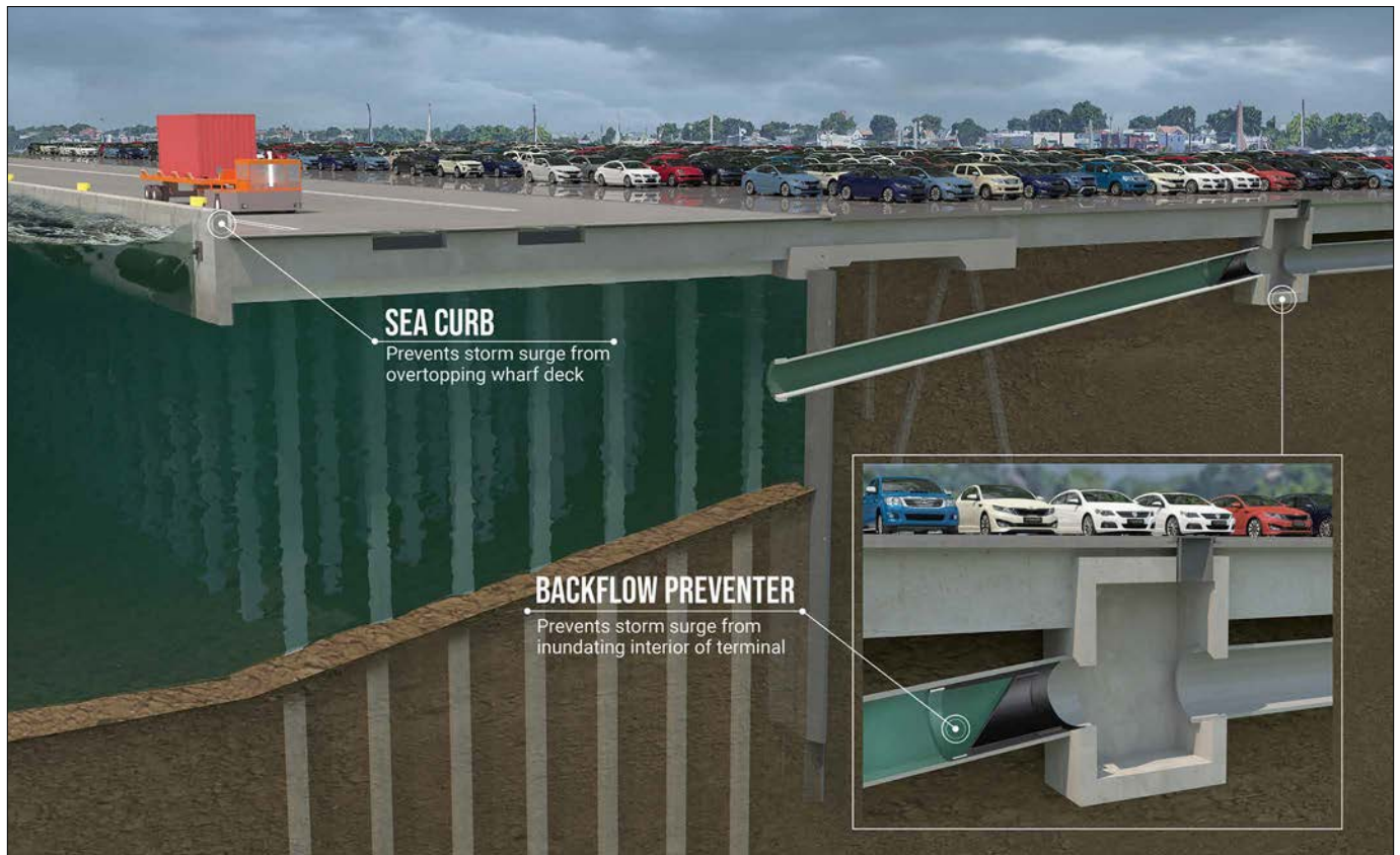
After Hurricane Isabel flooded the Port of Baltimore's Dundalk Marine Terminal and downtown Baltimore in September 2003, the Port of Baltimore developed a project to provide flood mitigation improvements at terminal. The project includes a perimeter barrier to prevent overtopping, a box culvert with pump, and a series of backflow preventers in drains. The project is supported by a U.S. Department of Transportation grant and administered by MARAD. Photo courtesy of the Port of Baltimore.
