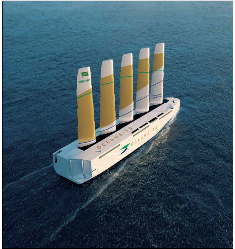
The Oceanbird , by Wallenius Marine, is a 200-meter-long car ferry powered by rigid telescopic wing sails and is expected to set sail in 2024. Photo courtesy of Wallenius Marine
