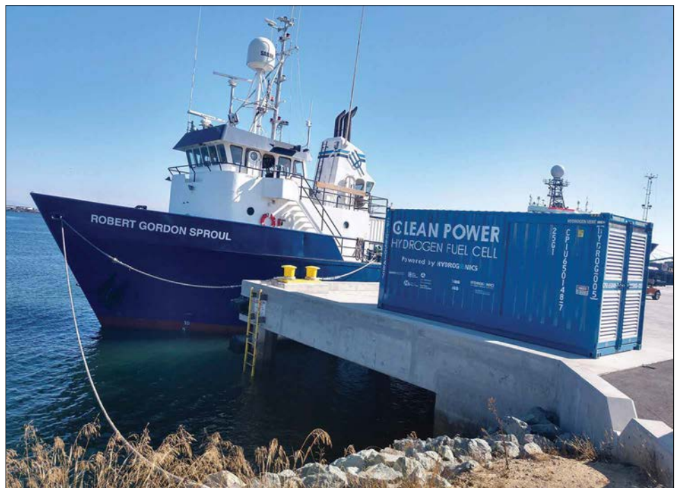
Scripps Institution of Oceanography is in the process of replacing the aging R/V Robert Gordon Sproul with a new hydrogen hybrid research vessel. The H_2 Hybrid SRV will use hydrogen in the form of a fuel cell generator, like the one seen here. Photo courtesy Bruce Appelgate, Scripps Institution of Oceanography
