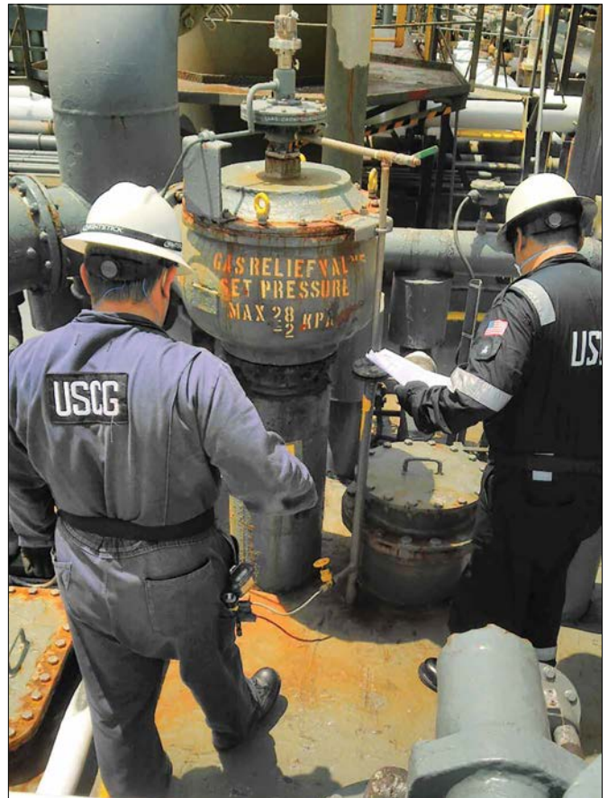
Coast Guard marine inspectors conduct examination of a cargo tank relief valve during a Liquefied Gas Carrier Accelerated Program course. Coast Guard photo
