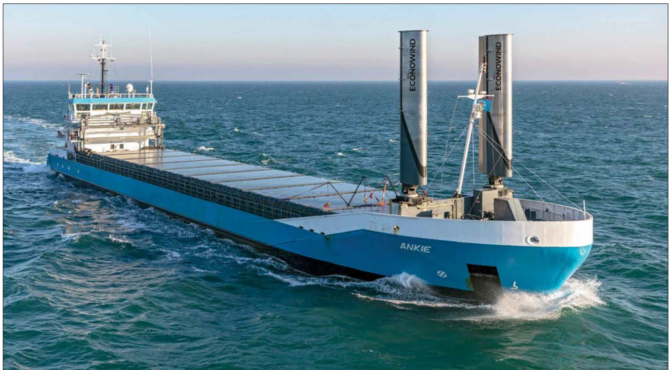
Two eConowind Ventifoils mounted on the bow of the M/V Ankie . Each sail is approximately 33.8 feet in height and uses programming and automation to find the best wind angles to reduce engine power. Photo courtesy of eConowind
