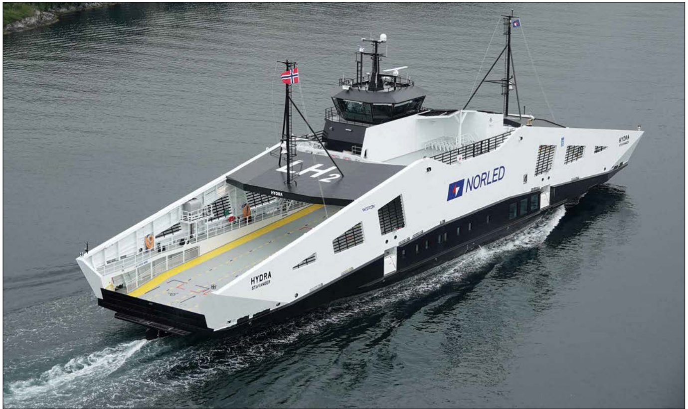
Owned by Norled, MF Hydra , the world's first hydrogen-powered ferry, has been operating between Hjelmeland, Skipavik, and Nesvik, on Norway's southwest coast under electrical operation, with hydrogen installation onboard expected in 2022. Photo courtesy of Norled
