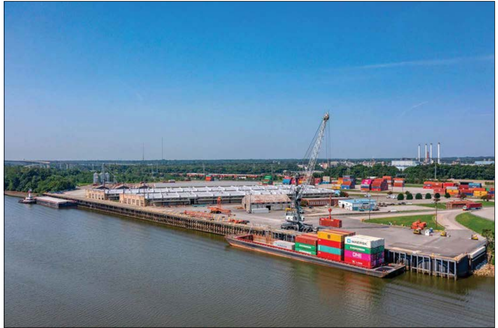
An inland terminal, the Port of Virginia's Richmond Marine Terminal, is served by a container-on-barge service from Hampton Roads along M-64, a marine highway route that removes container traffic from local roads and highways. Photo courtesy of The Port of Virginia
