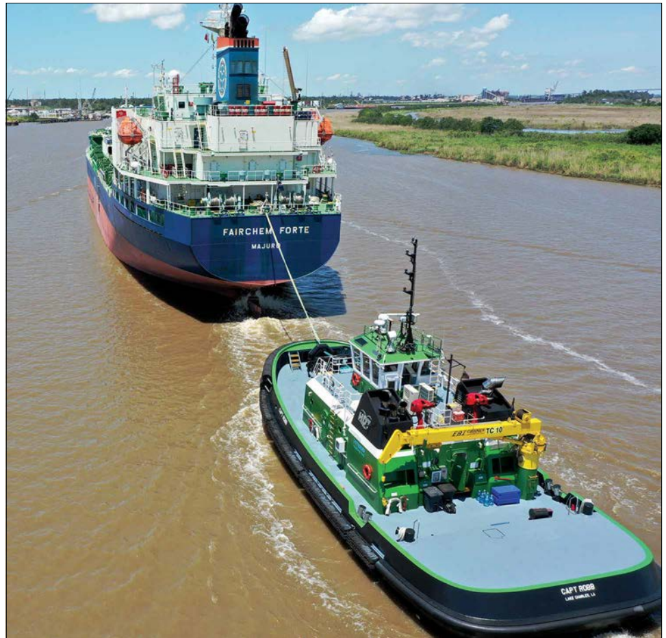
CAPT Robb, pictured here, and Ralph, are two of Harbor Docking and Towing's newest hybrid diesel-electric tugs. Built by Washburn & Doughty Associates Inc., they are 93 feet long, 38 feet wide, and boast 91 short tons of bollard pull. Each tug is powered by two 2,550 HP main engines, two 565 KW generators, and a 200 KW generator. Photo courtesy of Harbor Docking and Towing
