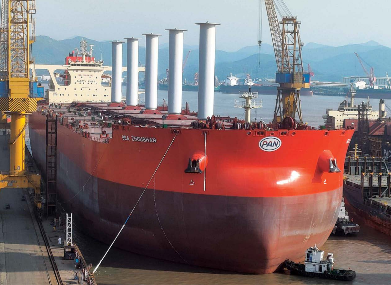
Ore carrier Sea Zhoushan is the latest vessel to be equipped with five Norsepower rotor sails. The project's goal is to reduce CO 2 emissions by 3,400 tons per year and increase the efficiency of the vessel's propulsion system by 8 percent. Photo courtesy of Norsepower Oy Ltd.
