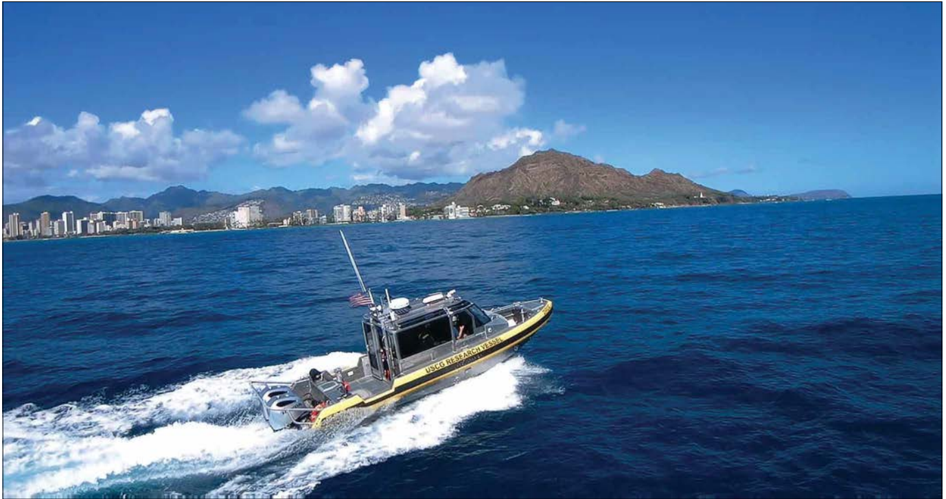
The 29RDC, a 29-foot autonomous vessel, conducts an autonomous mission off the Honolulu coast in November 2020. The USV was controlled by a laptop, but was also successfully remotely operated by Research and Development Center watchstanders in New London, Connecticut, 5,000 miles away. Coast Guard photo
