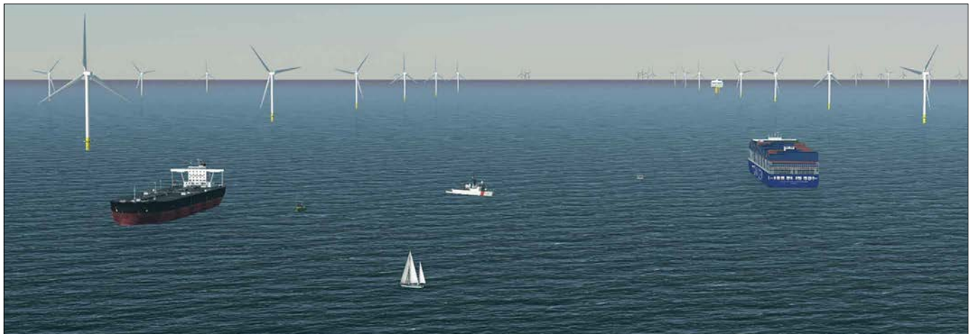
A scaled image from a full-size bridge simulation model of Ørsted's Revolution wind farm shows how vessel traffic would appear in a 1 nautical mile by 1 nautical mile area. Note there are multiple vessels in the image—including the largest container ship in the world—all within the 1 nautical mile width between turbines. Graphic courtesy of the U.S. Maritime Resource Center
