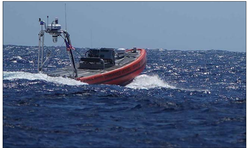
The Watcher is a Coast Guard cutter boat-large platform developed by Spatial Integrated Systems Inc. with solar arrays, a maritime domain awareness suite, and autonomy controls. This unmanned service vehicle was successfully tested in late 2020, and is a potential tool in the fight against illegal, unregulated, and unreported fishing in remote ocean areas. Coast Guard photo
