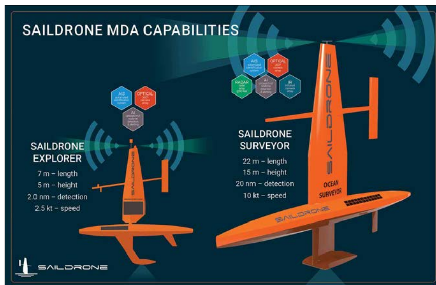
Saildrones' Generation 6 USVs are 23-foot long fiberglass sailing vessels with 15-foot fiberglass airfoil sails and feature onboard proprietary artificial intelligence software trained in vessel detection. Six of them participated in a 30-day maritime domain awareness demonstration period in late 2020. Graphic courtesy of Saildrone, Inc.
