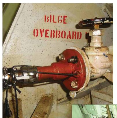
These images were part of the evidence submitted in the *B. Sky* case. Above: the bypass connection; Right: the bypass pump. Coast Guard photos
