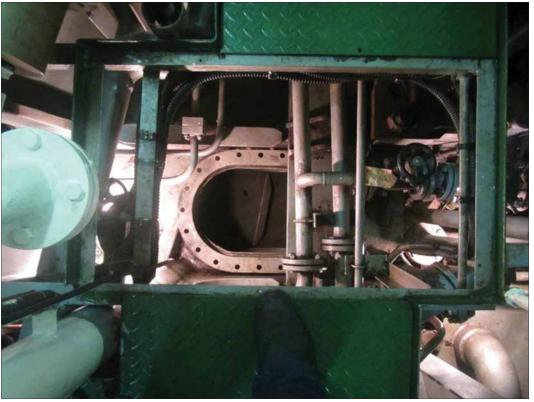
The B. Pacific's access hatch to the bottom void as found by Coast Guard investigators during expanded MARPOL exams. Coast Guard photo
