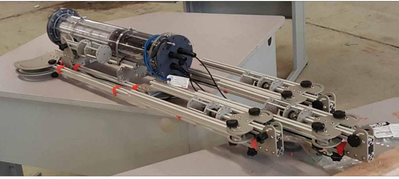
The Stevens Passive Acoustic Detection System (SPADES) can detect, track, and classify surface vessels. Stevens Institute of Technology graphic
