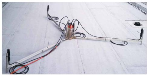
A Portable Acoustic Recorder System (PARS) is set up on shore before deployment. Stevens Institute of Technology graphic
