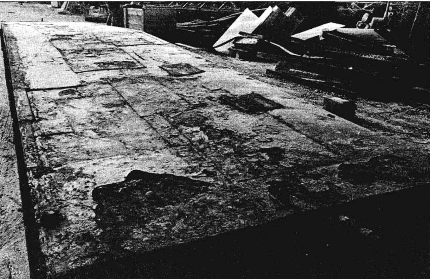
This forward panel on the No. 3 cargo hatch cover was removed from the *SS Marine Electric* in November 1982. This photo was taken in February 1983. U.S. Coast Guard photo.
