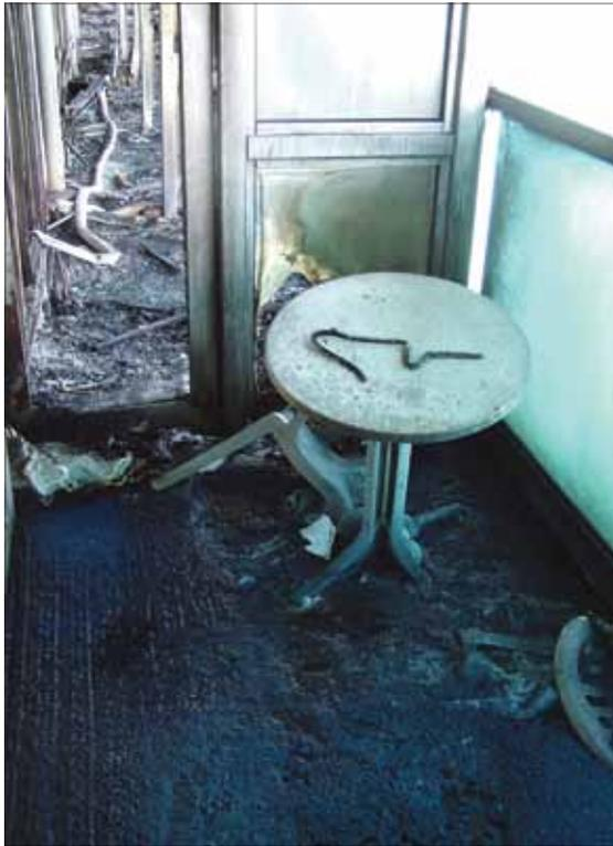
(Left) A *Star Princess* balcony before the fire. (Right) A corridor after the fire. (Below) The melted aluminium structure. Images courtesy of UK Marine Accident Investigation Branch.
