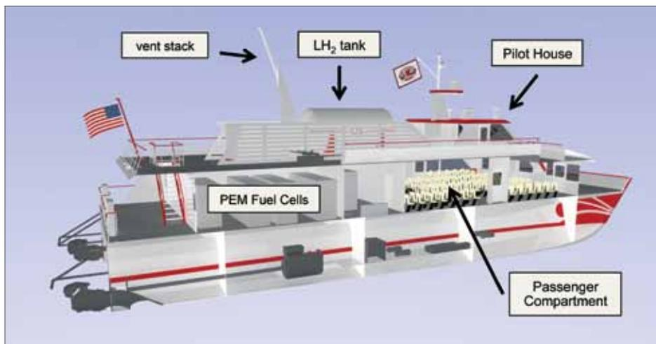
Engineering model of the *SF-BREEZE* as designed by Elliott Bay Design Group. The top deck holds the liquid hydrogen (LH<sub>2</sub>) storage tank, the associated vent stack, evaporation equipment, and the pilot house of the vessel. The main deck holds the PEM fuel cell power racks and the passenger compartment. Image courtesy of Sandia National Laboratories, from the Sandia Report SAND2016-9719, October 2016 (see bibliography).
