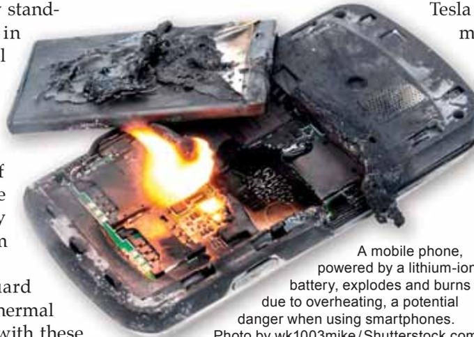
A mobile phone, powered by a lithium-ion battery, explodes and burns due to overheating, a potential danger when using smartphones.
