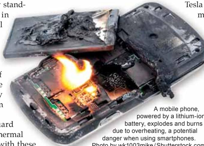
A mobile phone, powered by a lithium-ion battery, explodes and burns due to overheating, a potential danger when using smartphones. Photo by wk1003mike/Shutterstock.com.
