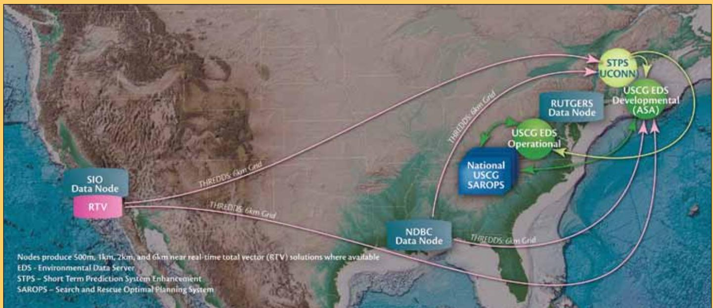
HFRNet data flow for ingestion into the Search and Rescue Optimal Planning System (SAROPS) tool. Image courtesy of SCCOOS.
