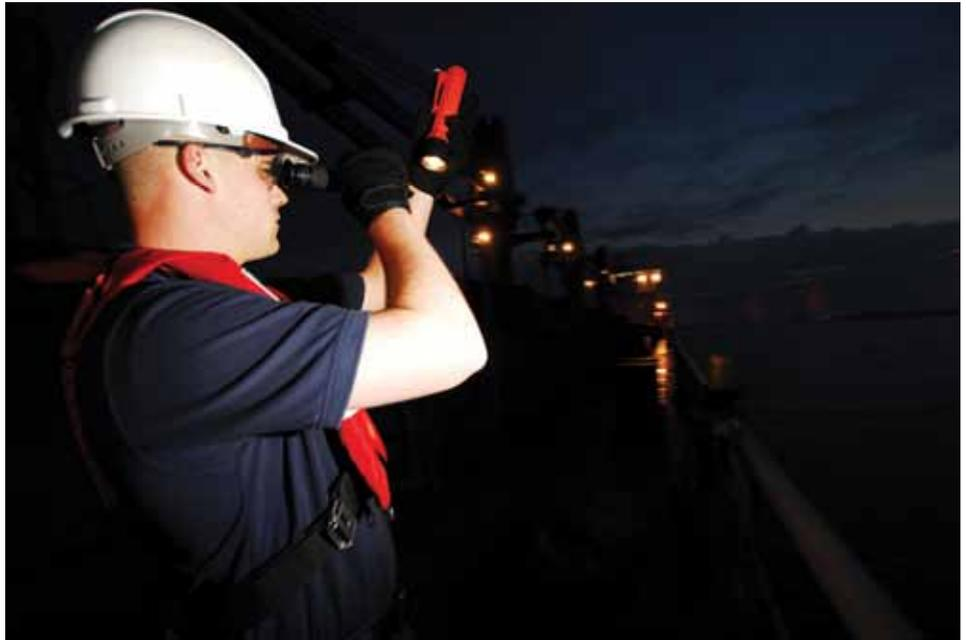
Petty Officer Travis Kelly, Marine Safety Detachment Massena peers at a sample of ballast water from the motor vessel Eider through a refractometer in Montreal. The U.S. Coast Guard inspects all vessels' ballast water before they enter the Great Lakes. U.S. Coast Guard photo by Petty Officer William B. Mitchell.
