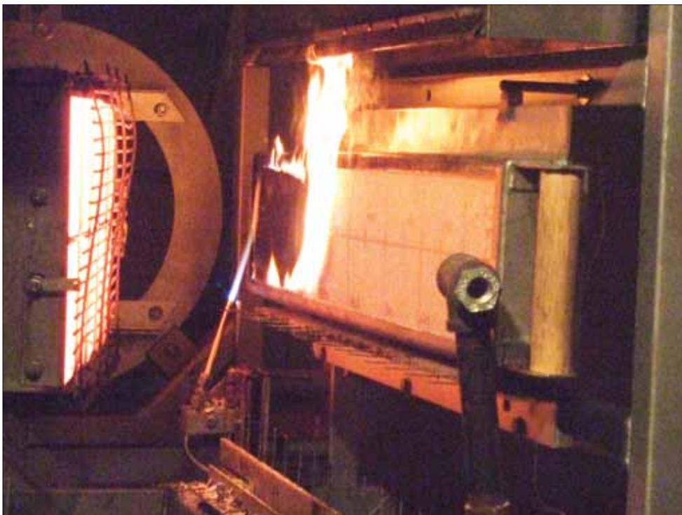
In this flame spread test, the specimen is tested for surface flammability (Part 5 of the IMO 2010 FTP Code). The flame is driven by the radiant panel on the left, which has been mounted at an angle to the specimen. U.S. Coast Guard photo by Mr. Louis Nash.
