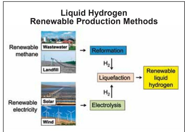
Example pathways for renewable (zero-GHG) liquid hydrogen production based on steam methane reforming, biomethane feedstock, or electrolysis of water using renewable electricity. Image courtesy of Sandia National Laboratories, from the Sandia Report SAND2016-9719, October 2016 (see bibliography).
