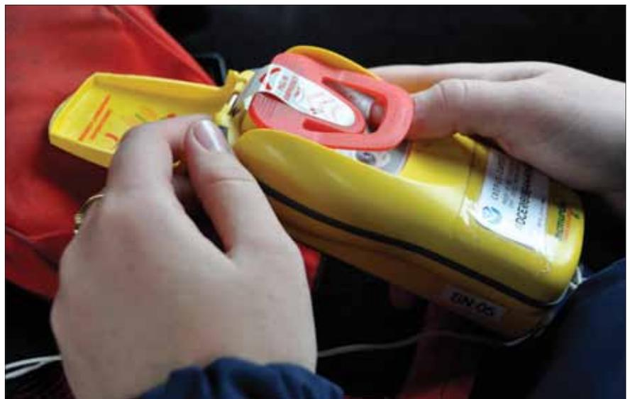
A personal emergency position-indicating radio beacon (EPIRB) can be attached to an individual, allowing the Coast Guard to identify and track the individual in a distress situation. U.S. Coast Guard photo by Petty Officer Barbara L. Patton.
