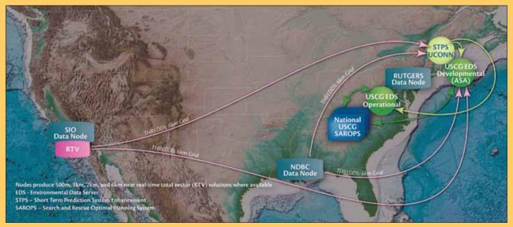
HFRNet data flow for ingestion into the Search and Rescue Optimal Planning System (SAROPS) tool. Image courtesy of SCCOOS.
