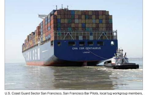
and CMA-CGM evaluate the capability of local tugboats to tow an ultra-large container vessel in the San Francisco Bay as part of an emergency towing operations preparedness drill. U.S. Coast to the issuance of the COI, although newly acquired vessels are granted up to six months of operation after the issuance of the initial COI in order to ensure full implementation of the system prior to vessel audits.
