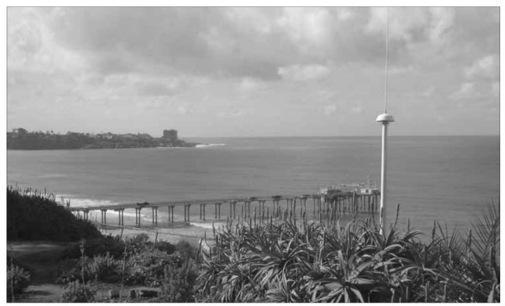
This "receive" antenna from a CODAR Ocean Sensor 5MHz SeaSonde system, installed at the Scripps Institution of Oceanography, La Jolla, California, is an example of a coastal installation. Photo courtesy of the Southern California Coastal Ocean Observing System (SCCOOS).
