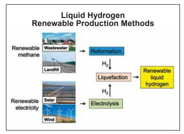
Example pathways for renewable (zero-GHG) liquid hydrogen production based on steam methane reforming, biomethane feedstock, or electrolysis of water using renewable electricity. Image courtesy of Sandia National Laboratories, from the Sandia Report SAND2016-9719, October 2016 (see bibliography).
