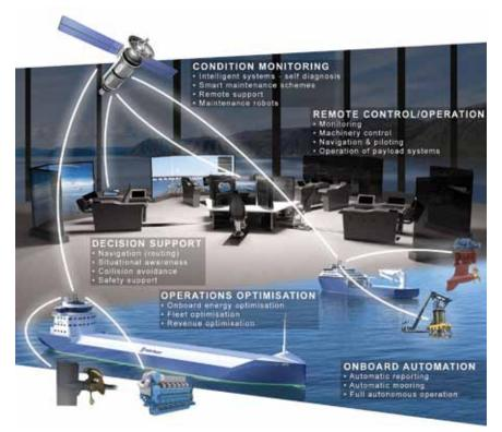
This figure depicts a conceptual design by the Rolls Royce Ship Intelligence Project which shows the level of automation and connectivity that will likely permeate all aspects of ship design and control in the future. Photo courtesy of Rolls-Royce Marine.
