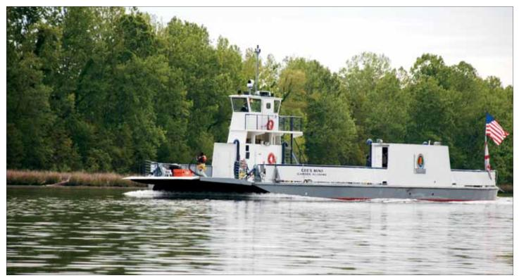
The Gees Bend ferry, operated by the Alabama Department of Transportation and Horn Blower Marine Services, is currently being converted into the first inspected, U.S.-flagged, all-electric, lithium-ion battery powered vessel. Photo courtesy of the Alabama Department of Transportation.
