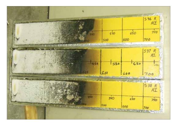
Specimens of paint after being tested to Part 5 of the 2010 FTP Code. The numbers indicate the distance from the left edge in centimeters. Extension of the flame is only measured along the centerline. U.S. Coast Guard photo by Mr. Louis Nash.
