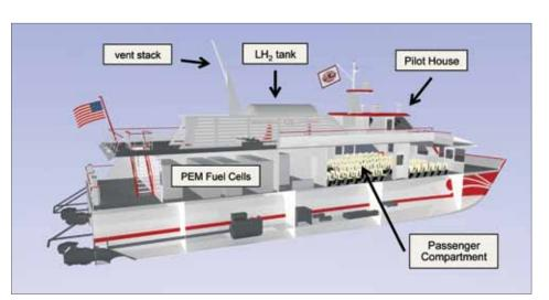
Engineering model of the *SF-BREEZE* as designed by Elliott Bay Design Group. The top deck holds the liquid hydrogen ( $LH_2$ ) storage tank, the associated vent stack, evaporation equipment, and the pilot house of the vessel. The main deck holds the PEM fuel cell power racks and the passenger compartment. Image courtesy of Sandia National Laboratories, from the Sandia Report SAND2016-9719, October 2016 (see bibliography).
