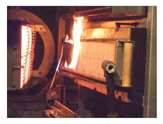
In this flame spread test, the specimen is tested for surface flammability (Part 5 of the IMO 2010 FTP Code). The flame is driven by the radiant panel on the left, which has been mounted at an angle to the specimen. U.S. Coast Guard photo by Mr. Louis Nash. no check for a material that produces a toxic gas that is not one of the listed gases.
