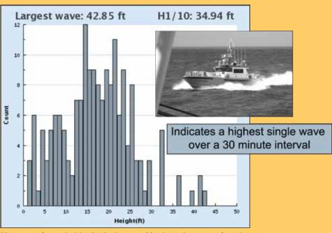
Histogram of wave height distribution over 30-minute time spans from the CDIP buoy at the mouth of the Columbia River, Pacific Northwest, United States. Graph courtesy of CDIP; photo courtesy of the Columbia River Bar Pilots.
