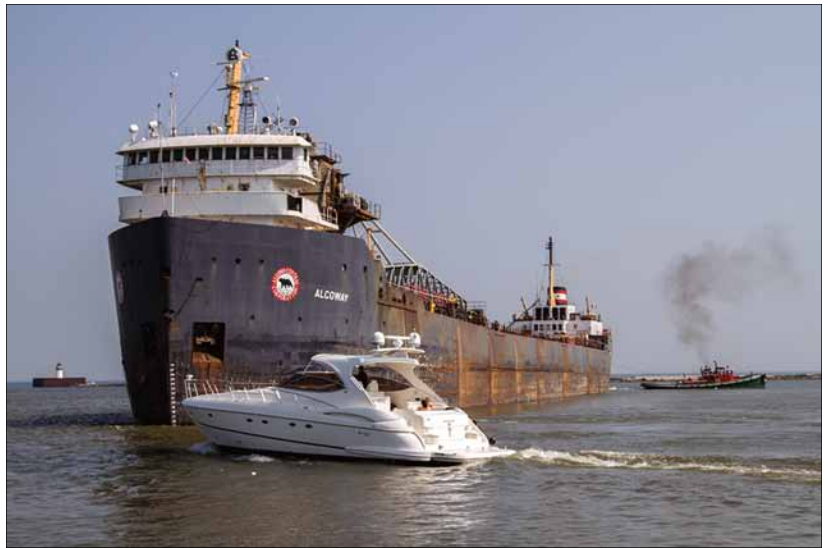
Recreational boat operating in unsafe proximity to the bow thruster and crossing too close to the bow while the vessel is underway. Photo courtesy of the Lake Carriers Association.
