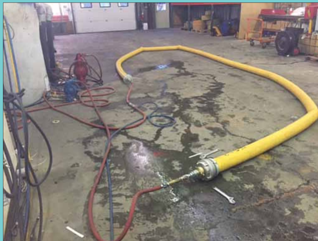
Every fuel hose is hydro-tested and inspected annually to ensure hose integrity. Picture courtesy of Mr. Greg Gladioux of Alaska Rubber.
