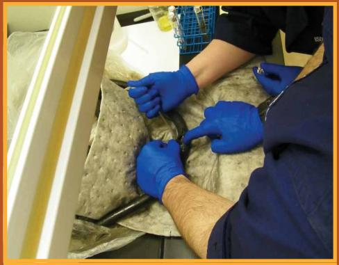
Marine Safety Laboratory personnel extract a sample from an oily water separator bypass hose, also known as a "magic pipe." Photos courtesy of the U.S. Coast Guard Marine Safety Laboratory.
