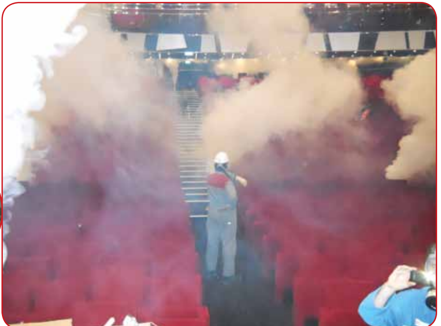
A theater is filled with smoke in preparation for the smoke extraction test.
