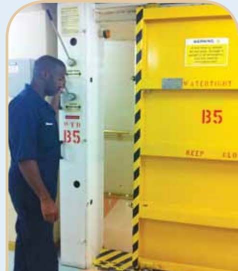
CWO Keith Macklin, USCG foreign passenger vessel examiner, observes watertight door testing.
