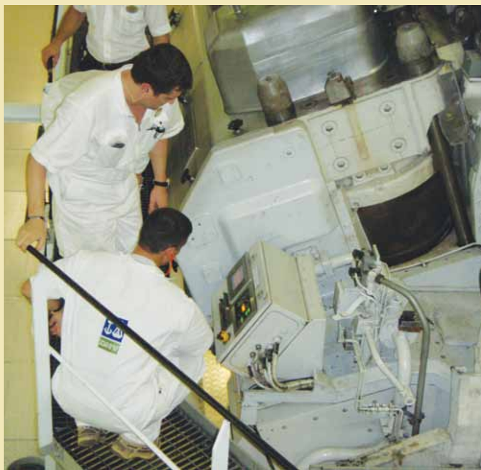
A surveyor witnesses main engine shutdown tests. All graphics courtesy of DNV GL.
