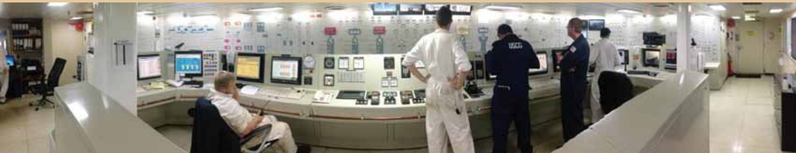
Mr. Brad Schoenwald and CWO Joseph Moskal, USCG foreign passenger vessel examiners, view a test of remote actuated valves. U.S. Coast Guard photos by ENS Jordan Ortiz.
