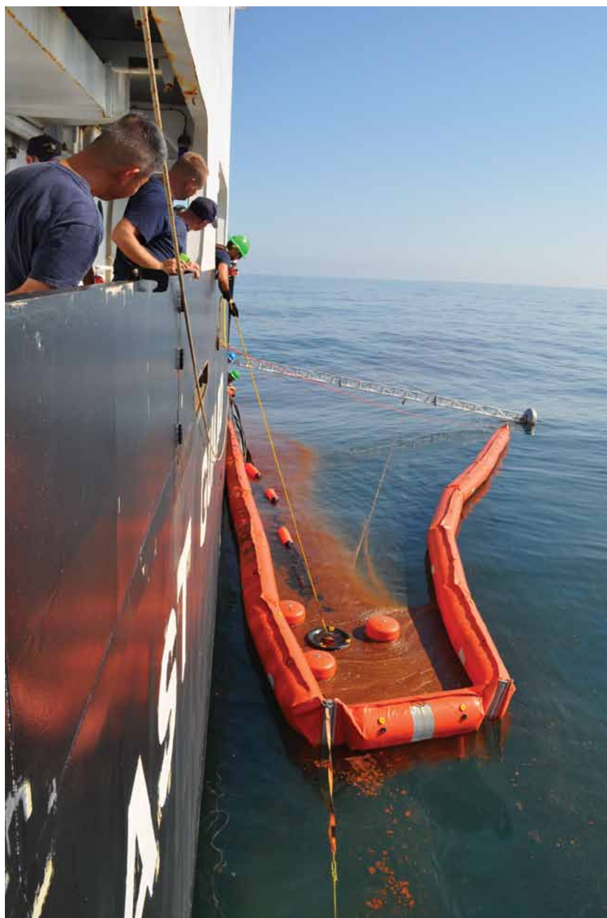
A Coast Guard Cutter deploys a skimming system. U.S. Coast Guard photo.
