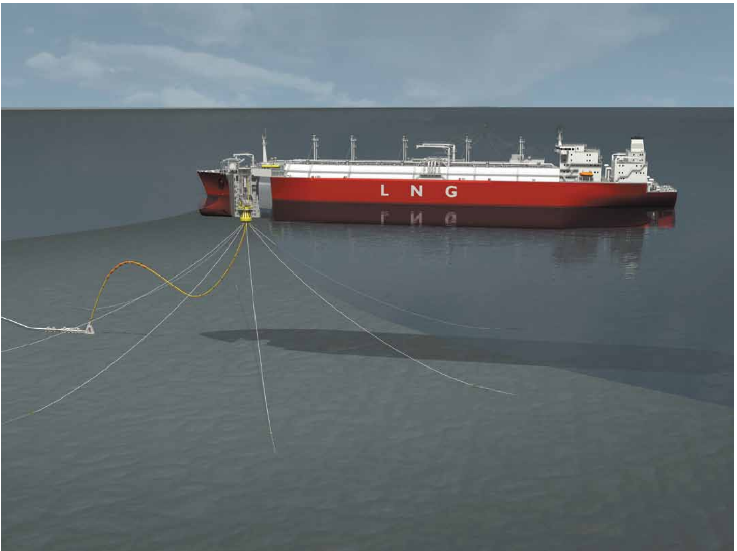
A liquefied natural gas regasification vessel prepares for transfer operations at a natural gas deepwater port. Image courtesy of Exceleerate Energy.
