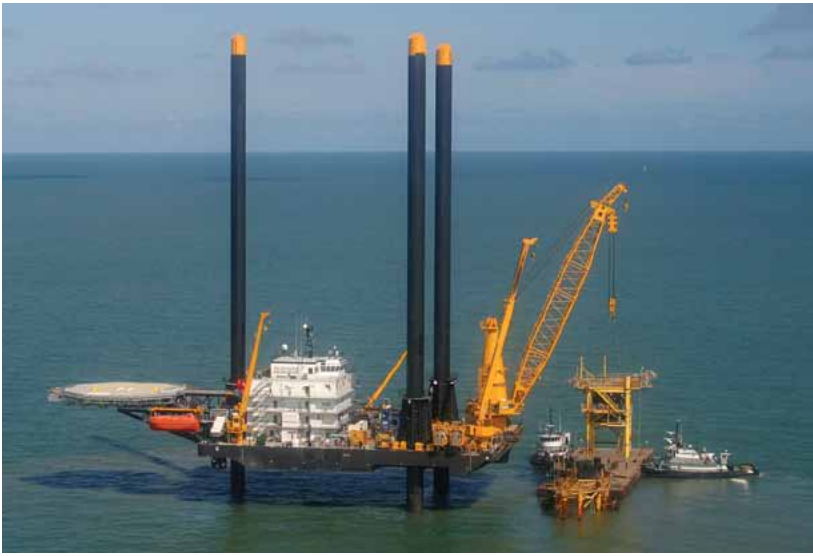
The 177-foot long, 3,915 GT liftboat Robert is a very large example of this special OSV class. Photo courtesy of Montco Offshore Inc.
