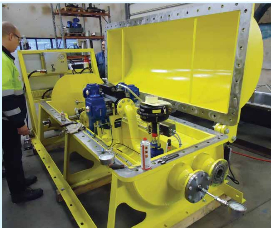
An ABS surveyor inspects a gas valve unit. U.S. Coast Guard photo by LT Chris Nichols.
