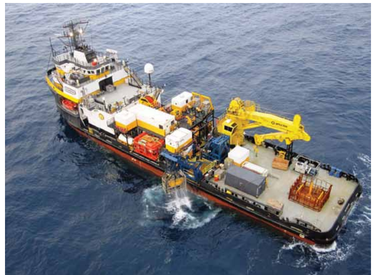
A diving platform vessel retrieves a remote operating vehicle.
