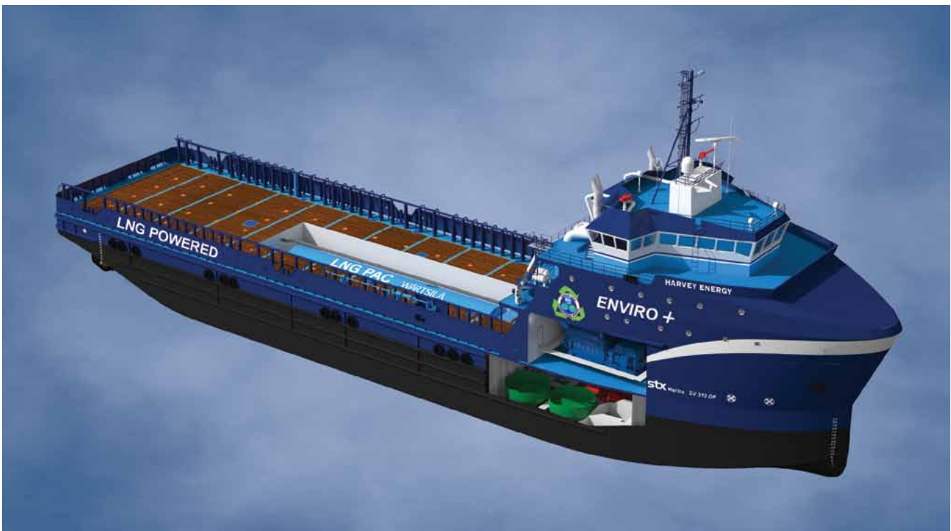
Conceptual graphic of the first U.S. OSV to use liquefied natural gas as fuel. Graphic courtesy of Harvey Gulf.
