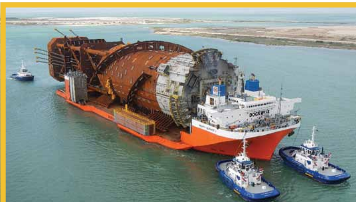
A spar arrives at the fabrication yard. U.S. Coast Guard photo by CWO Joel Smith.
