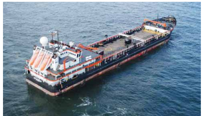
The 380-foot long multipurpose supply vessel HOS Centerline has its house in the aft part of the hull. Photo courtesy of Hornbeck Offshore Services.
