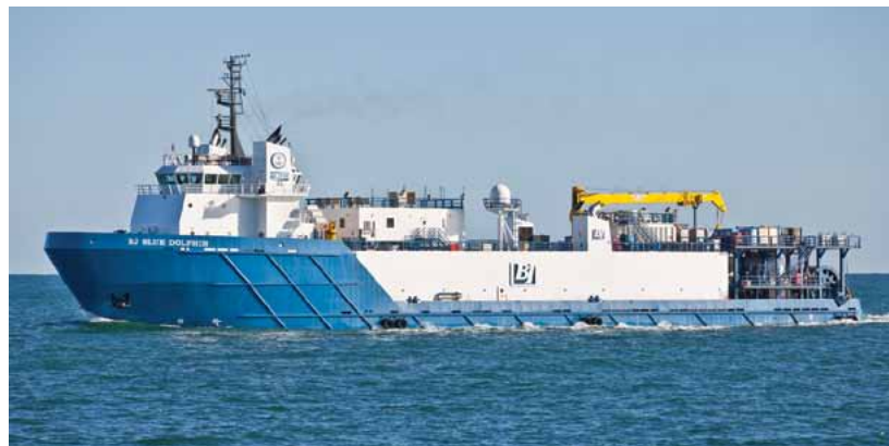
The 277-foot long well stimulation vessel Blue Dolphin . Note the absence of the aft open deck that typifies a conventional OSV. Photo courtesy of Edison Chouest Offshore.
