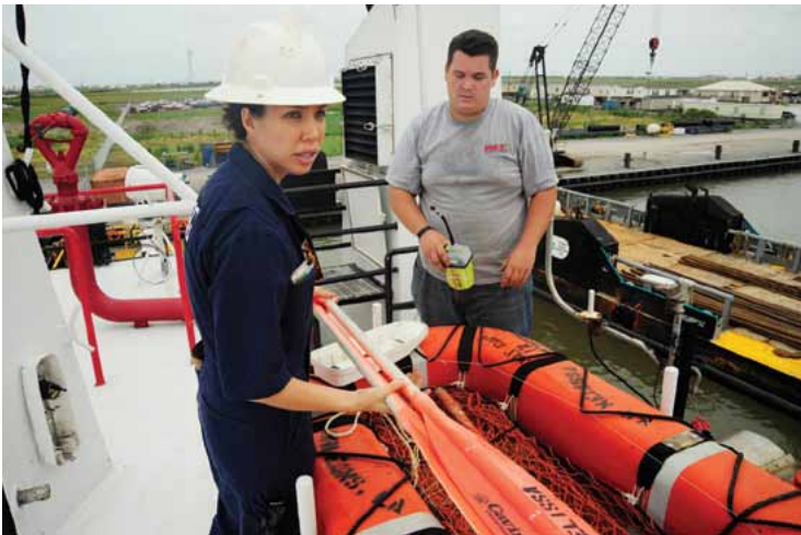
Lt. Sonha Gomez, a U.S. Coast Guard marine inspector, inspects a life float onboard an offshore supply vessel. U.S. Coast Guard photo by Petty Officer Ryan Tippetts.
