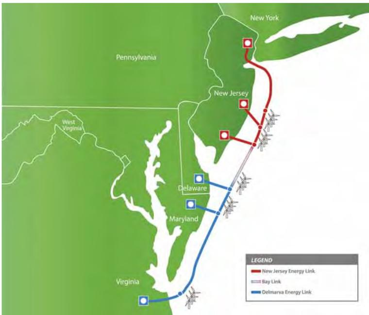
There will be six offshore platforms associated with the project, each capable of converting 1,000 megawatts of alternating current power (collected from the offshore turbines) to direct current power for delivery throughout the system.
