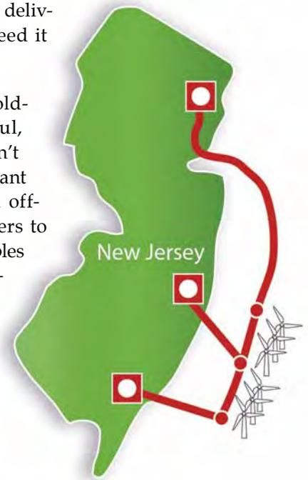
The first phase of the project will be the New Jersey Energy Link, which is capable of carrying 3,000 megawatts of offshore wind and delivering it to the strongest points on the terrestrial grid.
