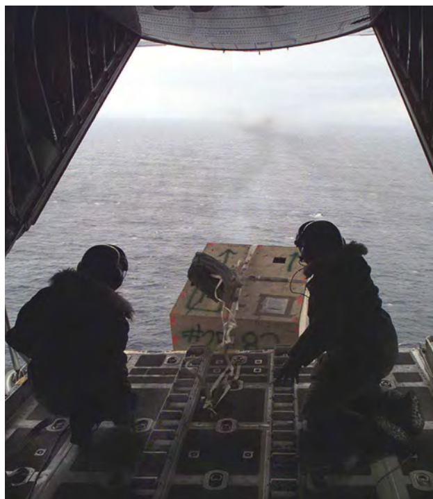
Aerial deployment of a World Ocean Circulation Experiment buoy, used to monitor ocean currents responsible for iceberg transport. USCG photo.
