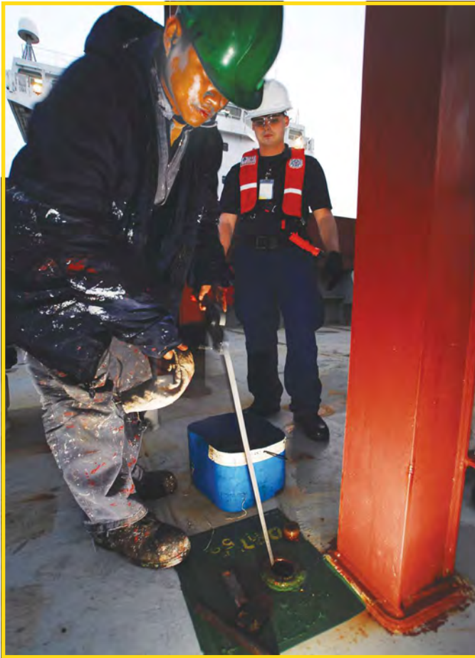
Ballast water sampling. The Ballast Water Convention is one of IMO's latest environmental protection measures. U.S. Coast Guard photo.
