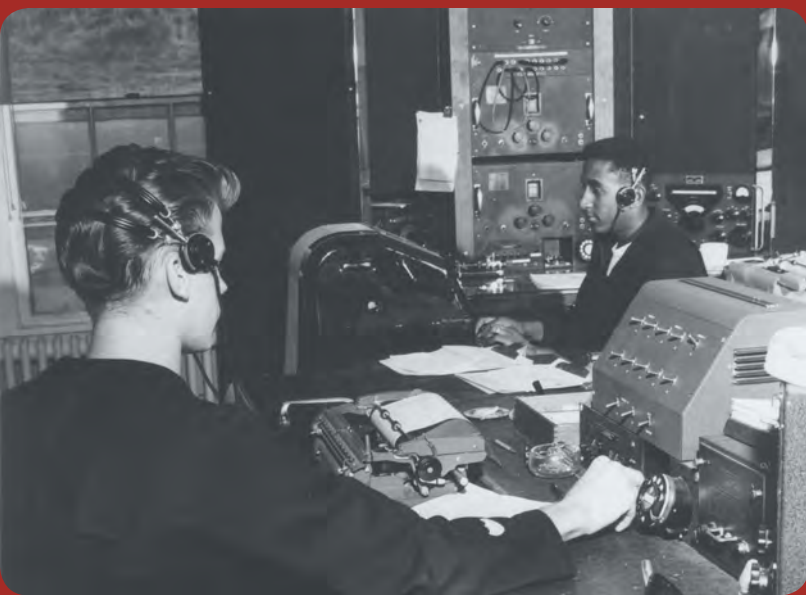
The position in the background is most likely the guard position, where an operator monitors 500 KHz continuously for distress, while processing more WDI 2 F RQ D Z RUNQJ I UHTXHQF 7 KH SRVWRQIQ WHI IRUJU URXCG VKRZ V D WDCV-mitter control device (the panel with the toggle switches and dial telephone pad) used to control the mode and frequency of the selected transmitter, and a device called a “whetstone machine,” used with the automatic keying machine.
