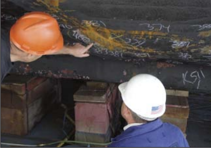
Vessel hull thickness is evaluated during an Alternate Compliance and Safety Agreement dry-dock examination. The examinations are conducted twice in every five-year period. USCG photo by Mr. Mike Rudolph.
