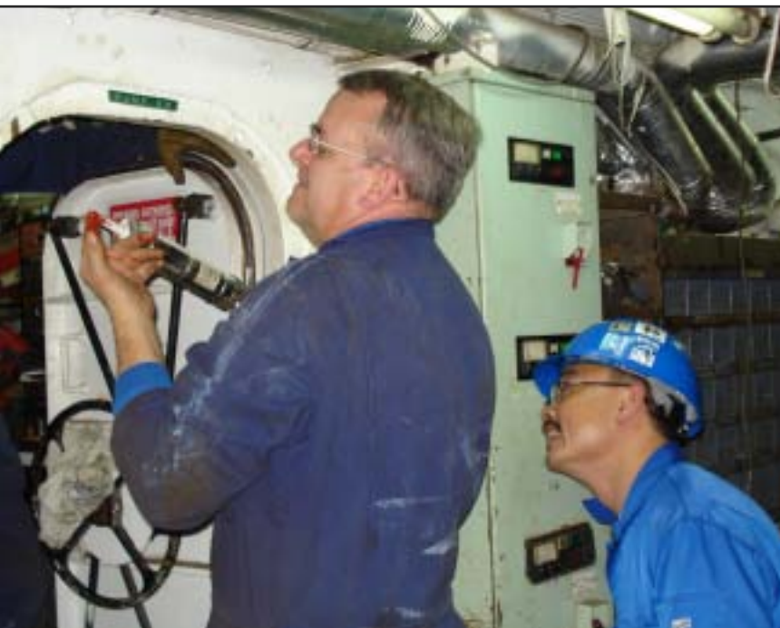
A U.S. Coast Guard marine inspector examines watertight integrity on a fish processing vessel. USCG photo.
