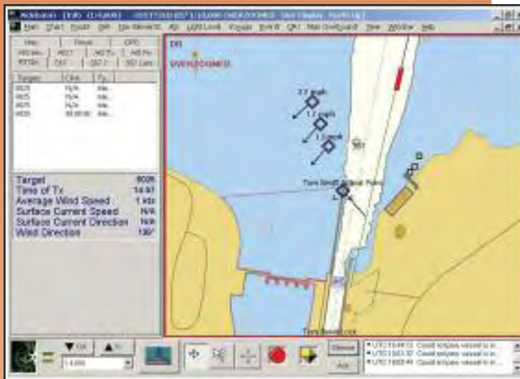
Outflow current velocity presented on an electronic navigational chart. The current data has been transmitted to the vessel via AIS.
