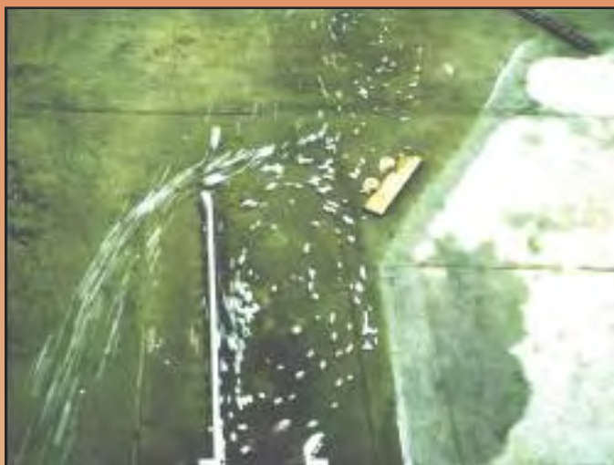
A model of the lock and dam shows the development of an outdraft current. Graphics courtesy of the U.S. Army Corps of Engineers.
