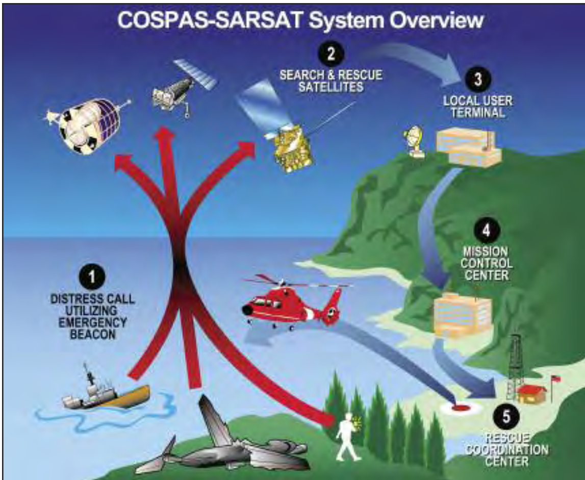
Cospas-Sarsat system overview. Graphic courtesy of the National Oceanic and Atmospheric Administration.
