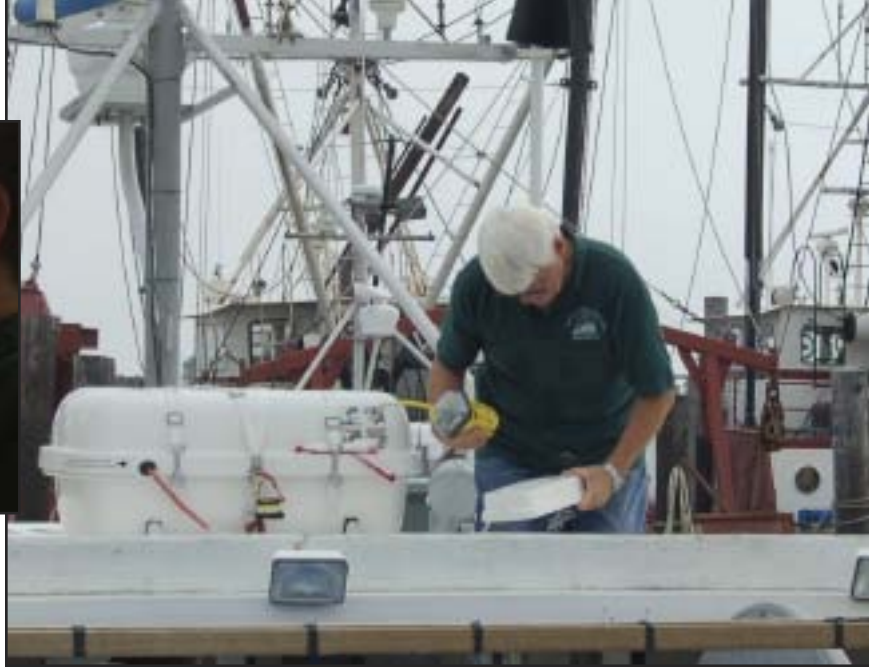
Figures 1 and 2: Coast Guard Auxiliarists check the safety decal affixed to the vessel after a satisfactory exam, and check the emergency position-indicating radio beacons and liferaft installed on the vessel as part of the safety exam. USCG photos.
