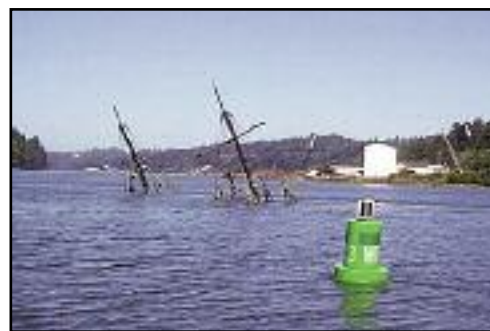
Figure 6: A foam buoy equipped with a self-contained LED light, marking a wreck in Yaquina Bay, Ore. Courtesy of www.solarmarinelights.com .
