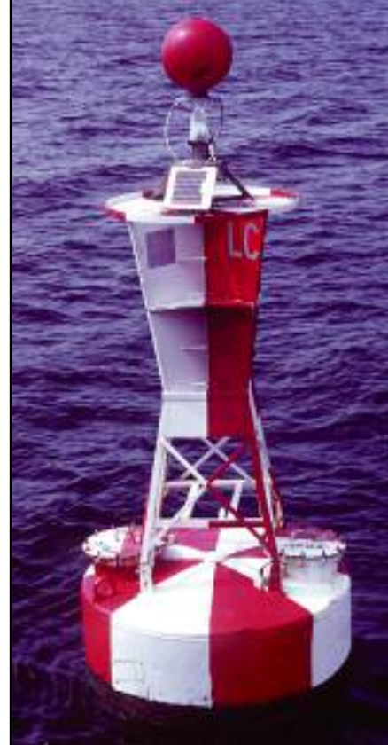
Figure 4: A solarized mid-channel buoy. Note the solar panels and single red sphere topmark. USCG photo.
