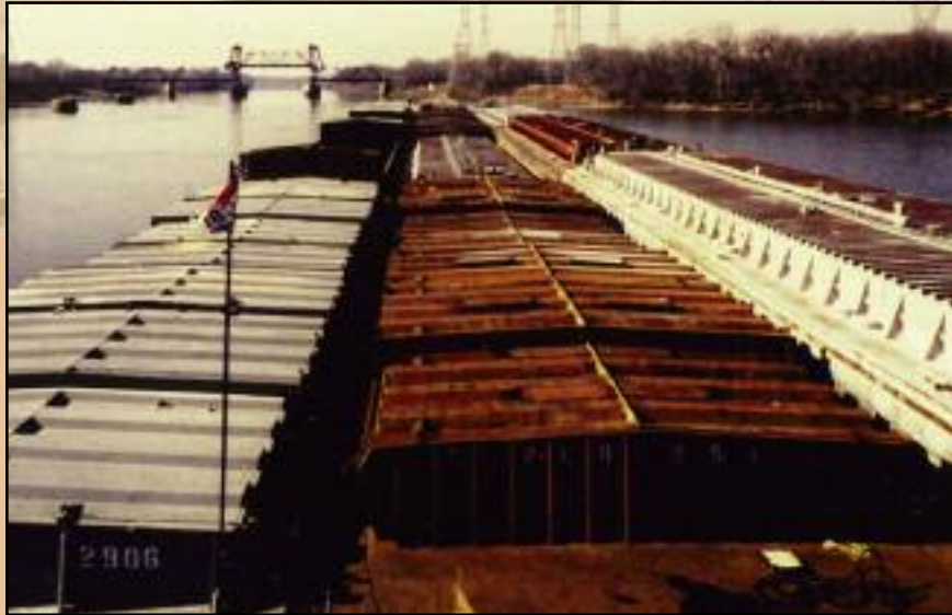
Figure 1: A southbound tow, 105 feet wide, approaches the Elgin, Joliet, and Eastern railroad drawbridge, located at mile 270.6 Illinois Waterway. The bridge features a mere 120.5-foot horizontal opening. USCG photo by W. F. Knutson.
