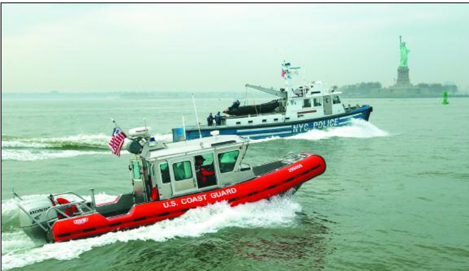
A 25-foot Coast Guard boat patrols the New York Harbor with a New York Police Department Harbor Unit boat. The Coast Guard's new 25-foot "Defender Class" boats can be equipped with heavier armament and can be transported by trailoring on highways or by air in C-130 aircraft. USCG photo by PA3 Mike Hvozda.
