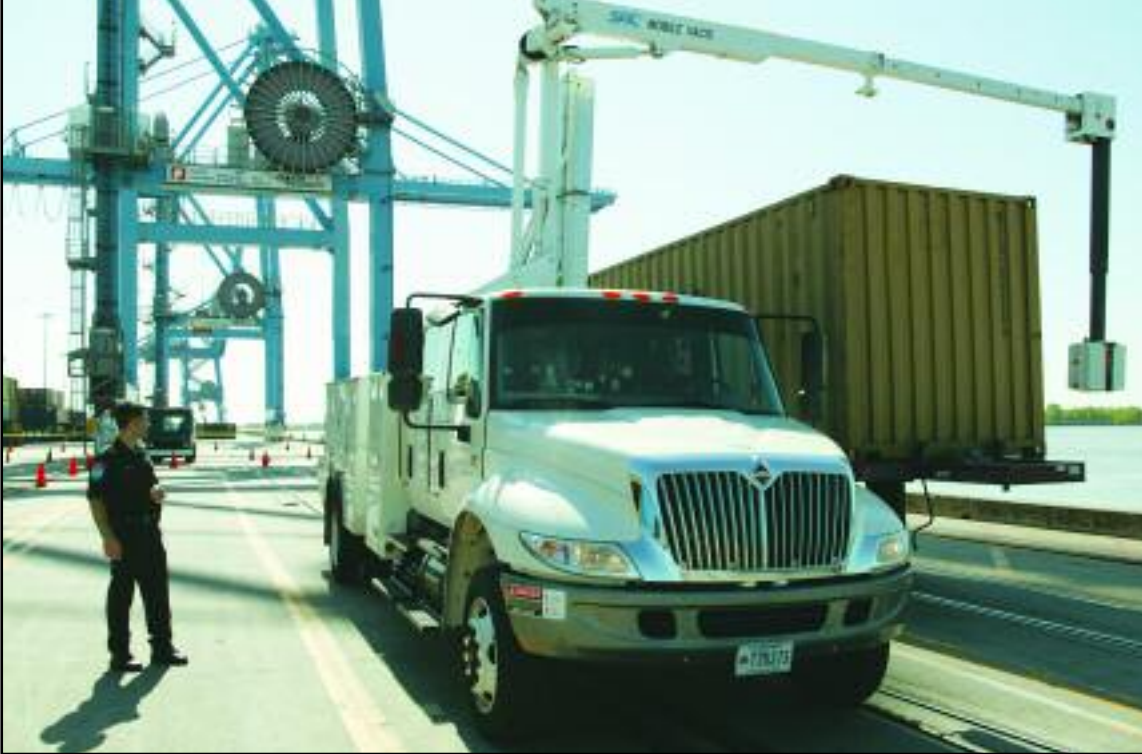
Figure 2: A mobile x-ray truck scans a container for contraband. CBP photo courtesy of Mr. James R. Tourtellotte.
