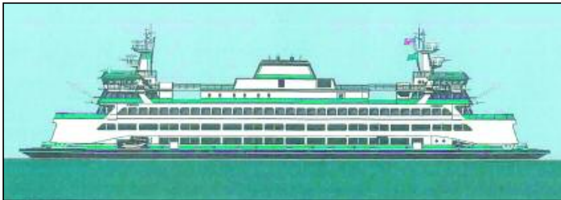
Figure 3: Drawing of the new WSF 130-auto, 1,200-passenger ferry. Drawing prepared by Gary Olsen, WSF Vessel Design.
