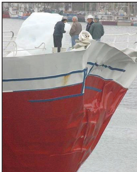
Figure 3. The Solborg sustained damage from a sizeable berg at least 50-65 feet high, off St. John's, in June 2004. Courtesy Keith Gosse, The Telegram, a division of Transcontinental Media Inc.
