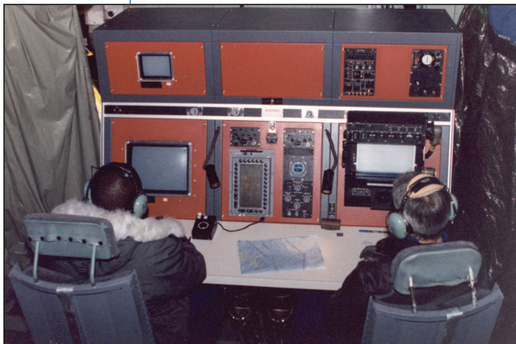
Figure 3: Radar Ice Observers use SLAR and FLAR to detect and classify targets on the ocean surface.
