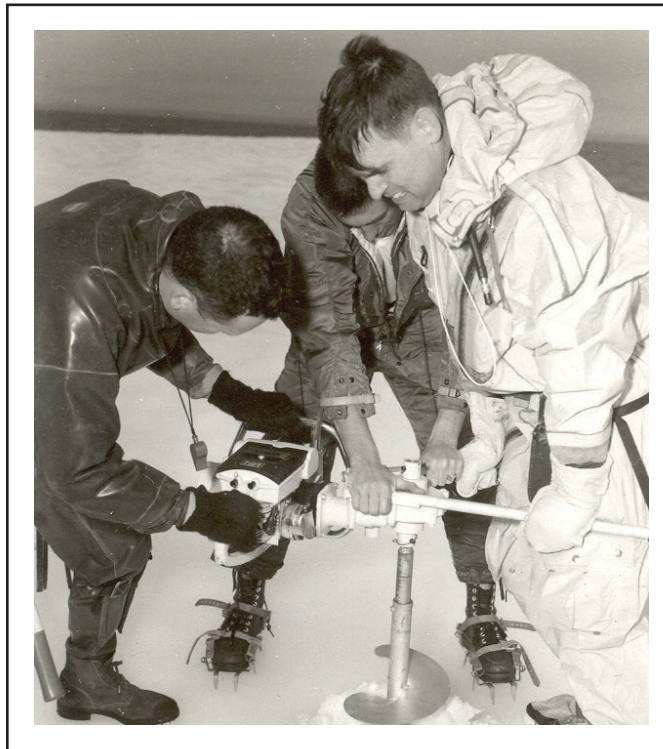
Figure 3: Drilling a hole in the iceberg with a power auger was a 45-minute procedure during the 1960 tests.
