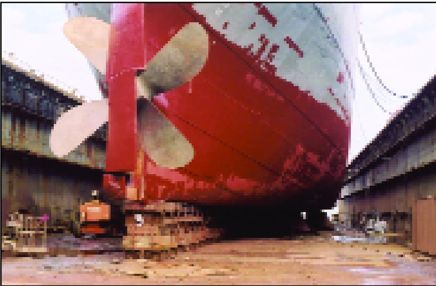
The John W. Brown was drydocked in October 2003 to satisfy Coast Guard hull inspection requirements. Louis Jerbi; courtesy Project Liberty Ship and SS John W. Brown .
