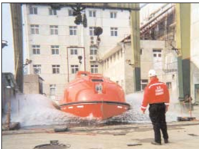
Lt. Madura witnesses a lifeboat drop test in Beihai, China. USCG photo.
