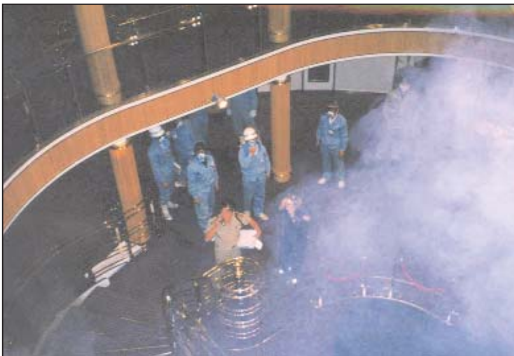
A smoke extraction test in the atrium of a cruise ship. USCG photo by Lt. Cmdr. John Mauger.
