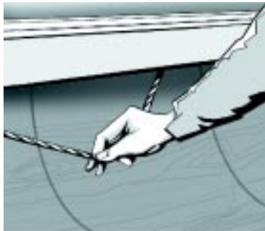
Figure 8. Gag line or kill switch for remote engine shut-off.
