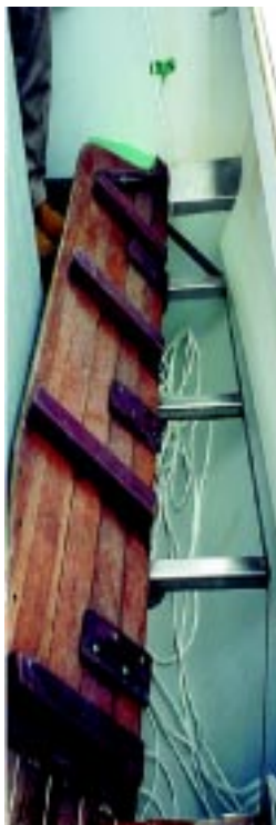
Figure 4. Rope locker (deck platform open) shows rope collecting under the deck away from the fisherman's feet.
