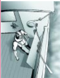
Figure 5. Rope bin made of plywood with a piano hinge that allows it to drop open and accept trap rope from the pot hauler.
