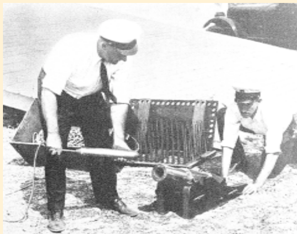
Coast Guards' line-throwing gun, shell, and line-box (June 1945).
