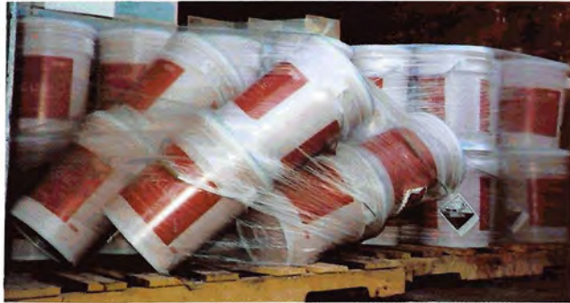
Improperly stowed drums of hazardous materials
