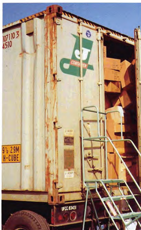
There was no blocking or bracing in a truck containing class 1.4 explosives.
