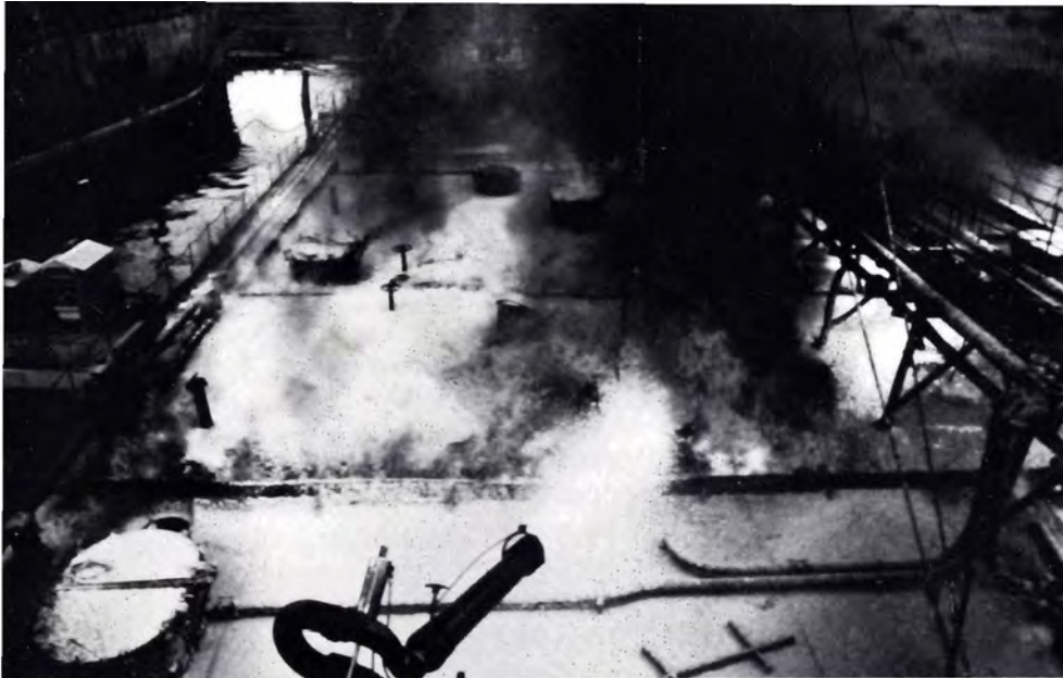
Monitor spreads foam on tanker deck fire.
