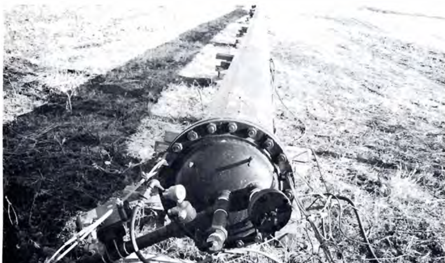
As far as the eye can see -- detonation arrester test piping can stretch a thousand feet.
