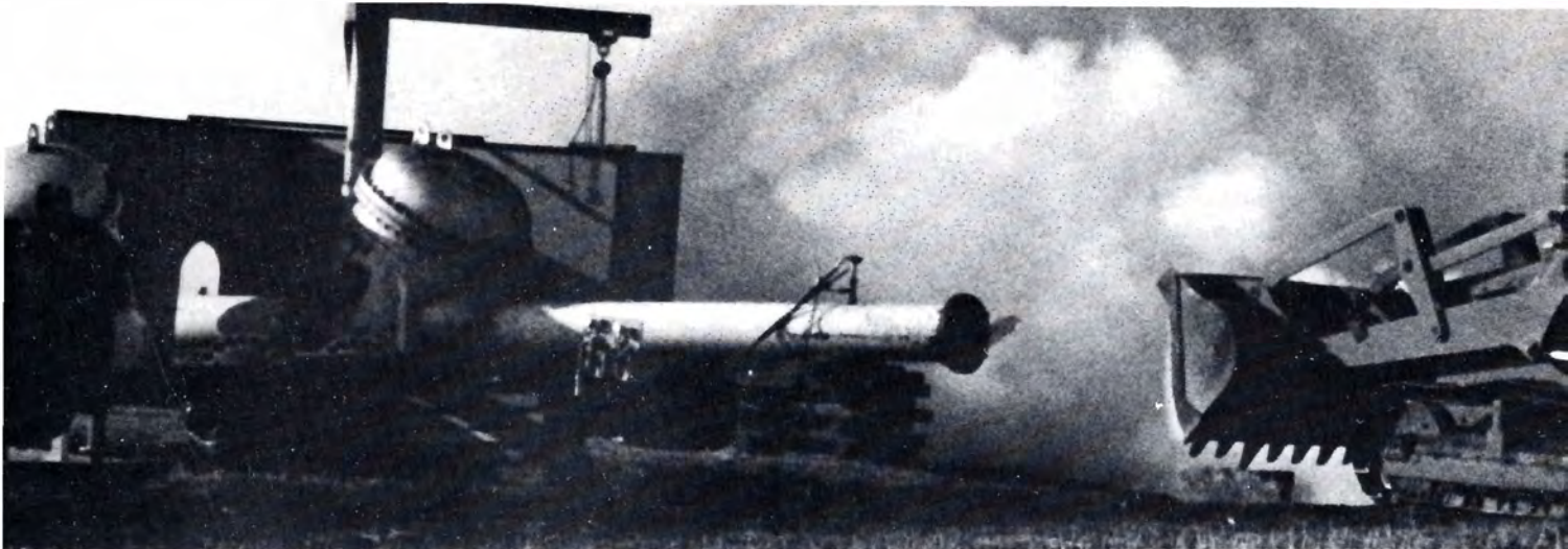
Detonation arrester is successfully tested in Alberta, Canada. (Front-end loader at right deflects combustion gases.)
