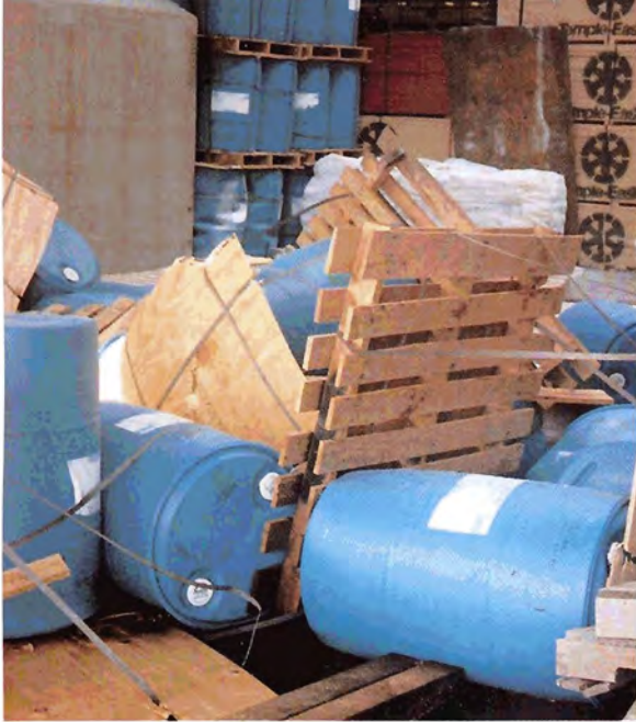
Improperly stowed drums of hazardous materials
