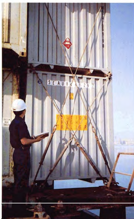
Coast Guard inspector verifies placement of flammables against vessel stowage plan.
