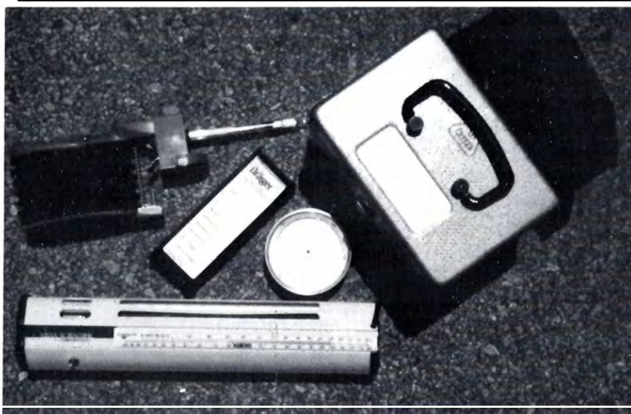
Coast Guard industrial hygienist sampling equipment includes colorimetric tube, pump, barometer and a device to measure relative humidity.
