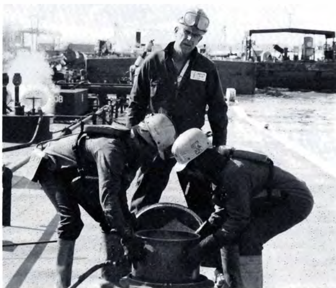
Marine chemist supervises checking of ventilation of cargo tank prior to testing and entry.
