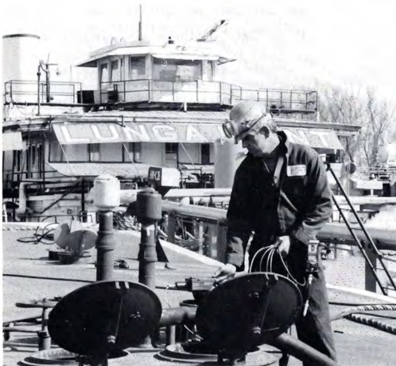
Marine chemist tests cargo tank for toxic atmosphere with an MSA photon gas detector.
