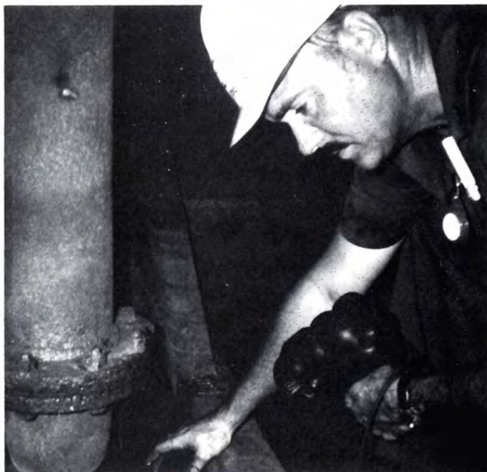
Marine inspector is monitored for benzene exposure during internal examination of cargo tank. Note passive organic vapor monitor hanging from his belt.
