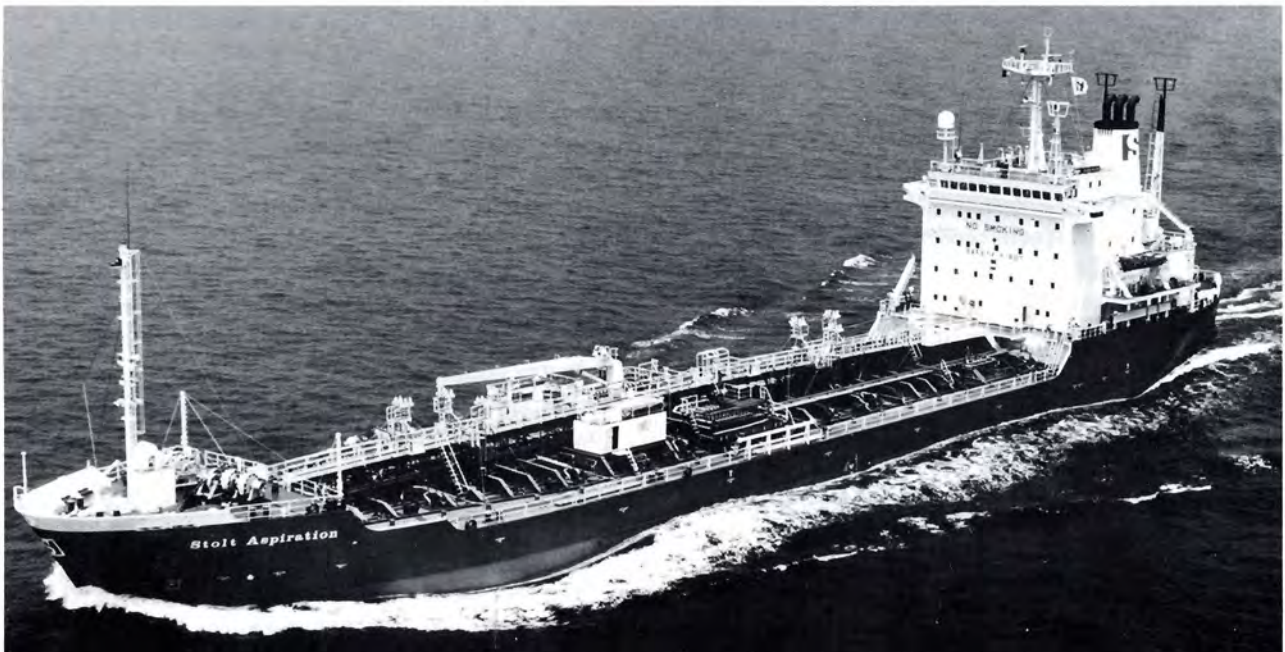
M/T Stolt Aspiration, 12,009 dwt medium-size parcel tanker, carries a variety of bulk liquids, including chemicals. Marine chemists must keep its spaces safe for shipyard "hot work" and inspections.
