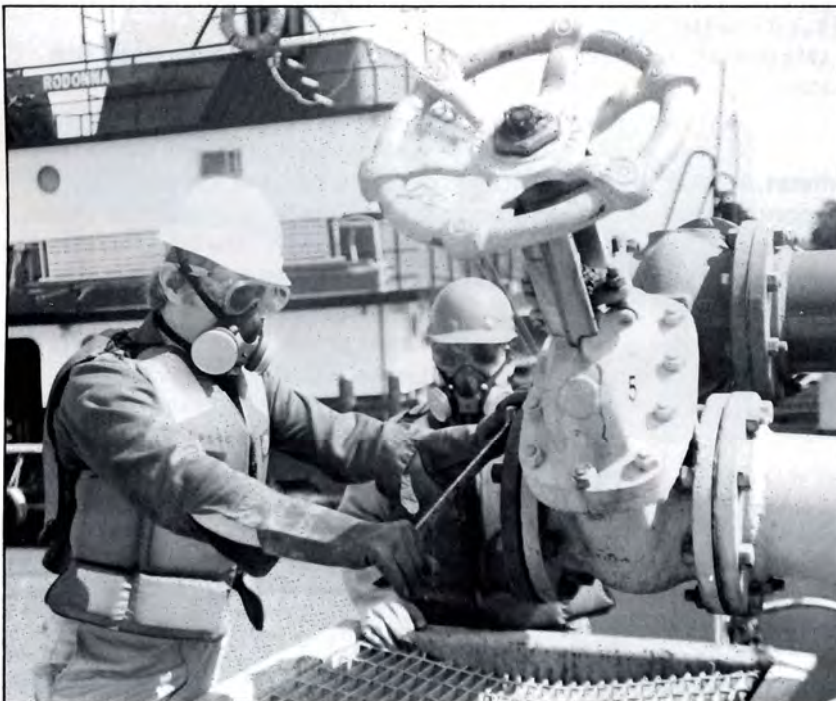
Tankerman demonstrates how to secure a liquid cargo transfer line.
