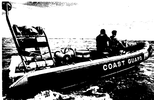
The cage over the Arctic 24's engine holds a gas-actuated system which will right the boat within 15 seconds of a capsize.
