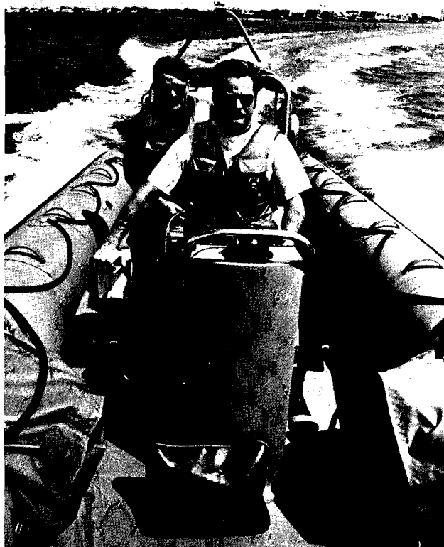
The Arctic 24 would hold 15 people and a third crewman in addition to the two shown above. The grablines along the sides of the boat are for people in the water.
