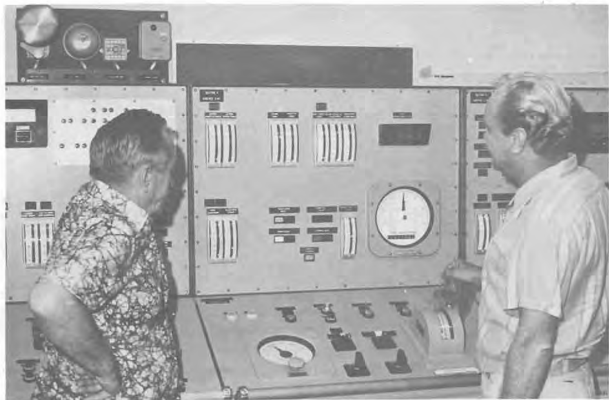
Student engineers in the applied electronics course operate the propulsion section of a ship's engine room console.
