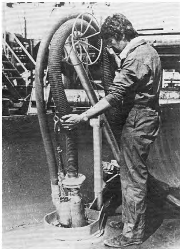
FRAMO model TK4 portable, hydraulic driven, submersible pump being inserted into a tank. This pump compares closely with those used extensively by the USCG National Strike Force.
